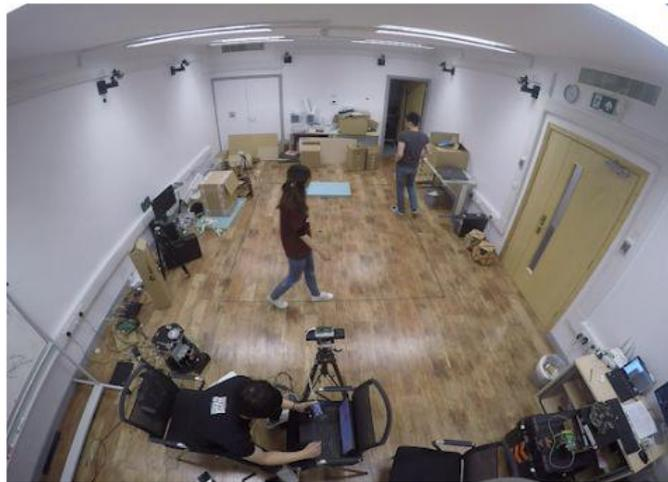
**Figure (19): Experiment Setting. "Vicon tracking system" used for collecting ground truth trajectories.[2]**
