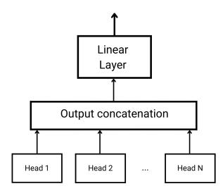
**Figure 4.4:** How the output of the GATv2Conv Layer is handled. If the layer has N attention heads, their output is concatenated into  $N*output\_channels$  array. This vector is passed to a Linear Layer which has an output size equal to output\\_channels dimension.
