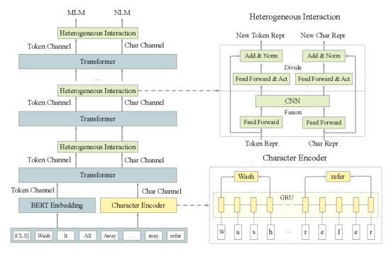
**Figure 3.8:** Architecture of the CharBert model [13], with focus on the *Character Encoder* and *Heterogeneous Interaction* modules.
