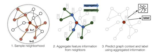
Figure 3.11: Examples of sampling and aggregation step from "Inductive Representation Learning on Large Graphs" [20]. Here k represents the number of layers of the model, which is linked to the depth of the neighbourhood, for example, k = 1 means that only direct neighbours are considered
