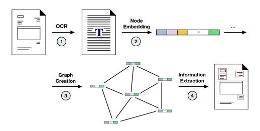
Figure 4.1: Graphical representation of the pipeline divided into steps. Step 1: The OCR tool docTR extracts text along with bounding boxes. Step 2: The text, along with the spatial features are used to create the node embeddings. Step 3: The graph is created using the Euclidean distance among nodes to select the edges. Step 4: Finally the graph is passed as a data point to the Graph Neural Network to extract the entities.
