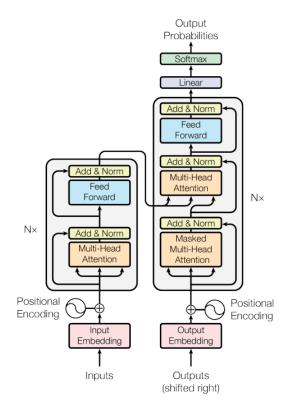
**Figure 3.5:** Architecture of the Transformer model [12], composed of their characteristic Encoder and Decoder modules, which both implement Multi-Head Attention.
