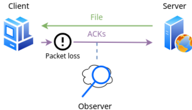
Figure 5.2: Traffic flow of a download with packet loss at the client.
