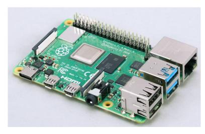
Figure 2.3: Raspberry Pi 4 Model B [6].
