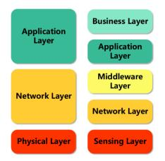
Figure 2.2: Three-layer and five-layer architectures [5].
