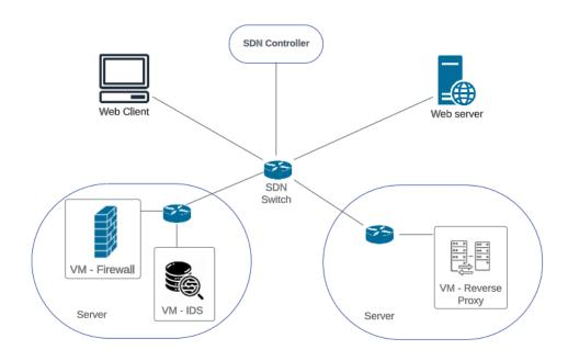
**Figure 3.7:** Example of a Service Function Chain Implemented with NFV and SDN technologies
