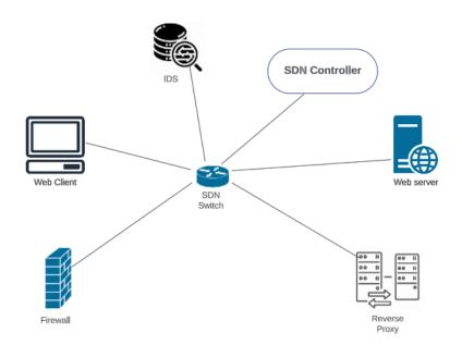
Figure 3.6: Example of SDN applied to a Service Function Chain
