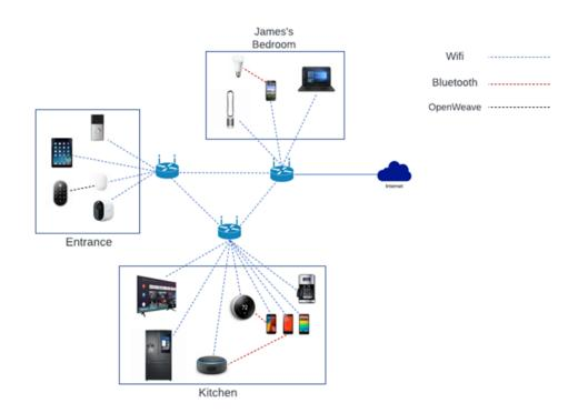
Figure 3.2: Overview of the different connections among the devices inside the smart home environment
