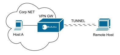
Figure 2.3. VPN model: Remote-connection
