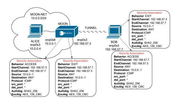
Figure 7.6. Testing Remote-Connection
