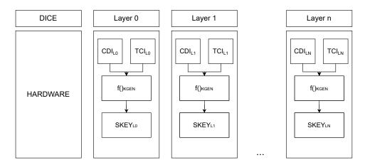
Figure 2.5. Symmetric key generation example (source: [4])
