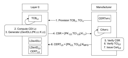
Figure 2.11. Example initial device identity (IDevID) certification by a manufacturer (source: [4])
