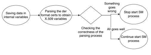
Figure 6.6. The initial operations at SM level
