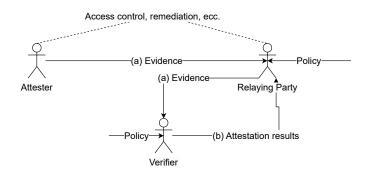
Figure 2.15. Role Interactions - Background Check Topology Model (source: [11])
