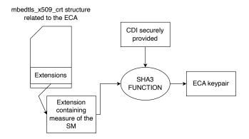
Figure 6.8. How the private key of the ECA keypair is calculated
