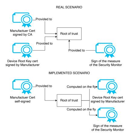
Figure 6.3. The real scenario vs the implemented scenario
