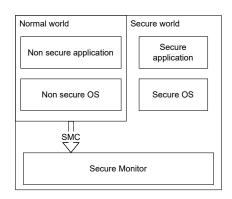
Figure 3.5. Interaction from the normal world to the secure one (source: [13])
