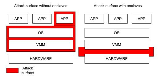
Figure 3.7. Comparison of attack surface between application running with and without SGX enclaves (source: [22])
