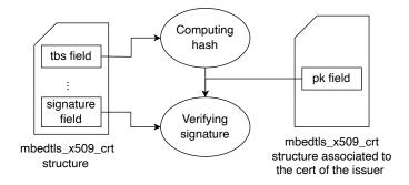
Figure 6.7. How the signature verification process works
