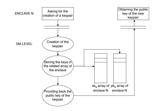
Figure 6.10. Creation of a keypair for a specific enclave
