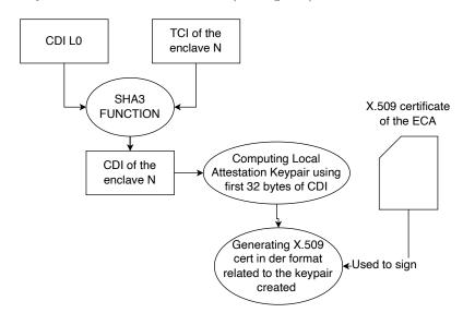
Figure 6.9. Computing the CDI of the enclave and its Local Attestation key
