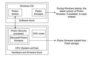
Figure 3.17. Pluton architecture (source: [34])
