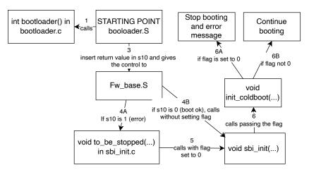
Figure 6.4. Secure boot flow
