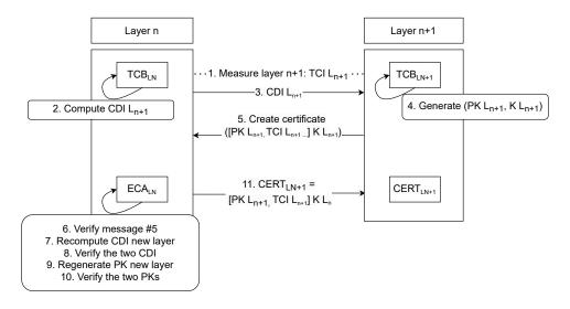
Figure 2.10. Layered TCB Certification using a CSR (source: [4])
