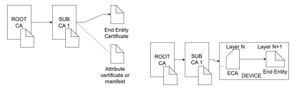
Figure 2.6. Certificate hierarchy with Attribute Certificate or Manifest and Certificate hierarchy with Embedded CA (source: [4])
