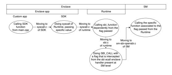
Figure 5.4. The communication flow between the EApp and the SM
