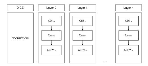
Figure 2.4. Asymmetric key generation example (source: [4])
