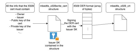
Figure 6.1. The flow to obtain a mbedtls\_x509\_crt variable
