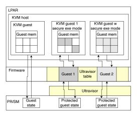
Figure 3.14. IBM Secure Execution protects guest memory and state (source: [24])
