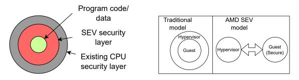
Figure 3.8. Security layers and SEV security model (source: [23])
