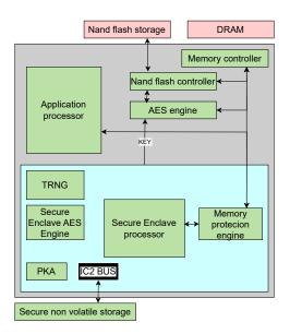
Figure 3.15. Overview of the secure enclave (source: [33])
