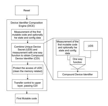
Figure 2.1. Compound Device IdentifierDerivation Process (source: [2])
