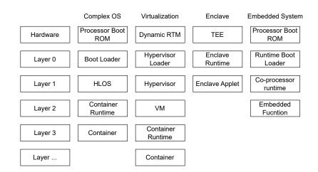
Figure 2.2. Examples of system layering (source: [4])
