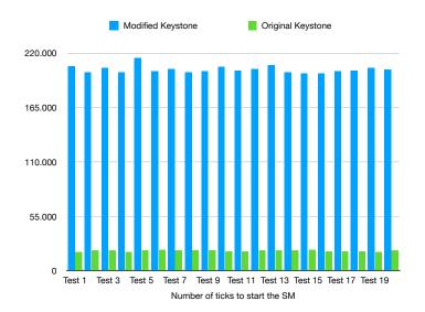
Figure 7.8. Comparison of the time needed to start the SM
