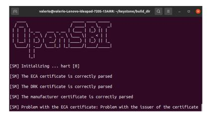
Figure 7.3. Failure during validating fields
