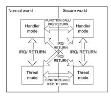
Figure 3.6. TrustZone on ARM cortex-M (source: [13])
