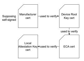
Figure 5.3. The chain from the Local Attestation Key to the Manufacturer cert (supposing it self-signed)
