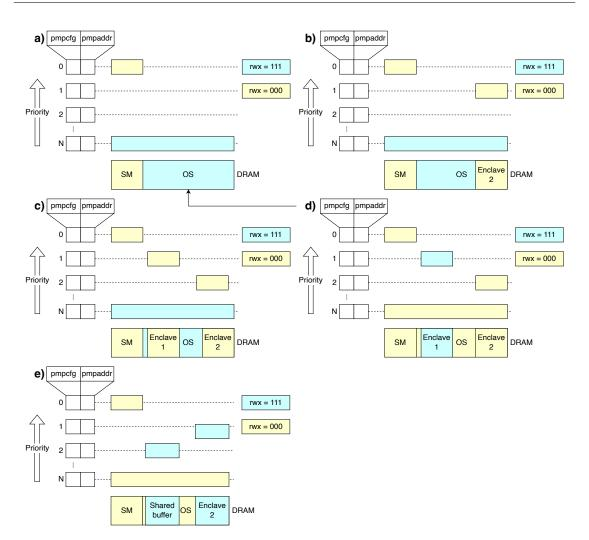
Figure 4.4. How Keystone uses RISC-V PMP for memory isolation
