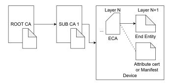
Figure 2.7. Certificate hierarchy with Embedded CA (source: [4])
