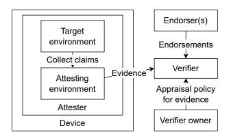
Figure 2.13. Device with Attesting Environment and Target Environment (source: [11])
