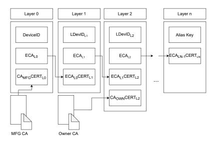
Figure 2.8. Layered certification example (source: [4])
