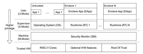
Figure 4.1. Different components in a system that implements Keystone enclaves (source: [25])
