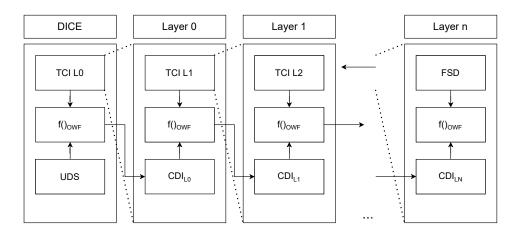
Figure 2.3. TCB layering architecture (source: [4])
