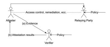
Figure 2.14. Passport Topology Model (source: [11])
