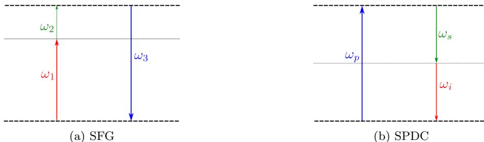
Figure 2: Sketch illustrating two three wave mixing processes : a) Sum Frequency Generation; b) Spontaneous Parametric Down Conversion
