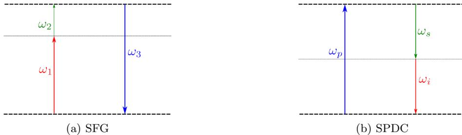
Figure 2: Sketch illustrating two three wave mixing processes : a) Sum Frequency Generation; b) Spontaneous Parametric Down Conversion
