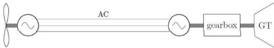
Figure 2.5: "Configuration Diagram Turbo Electric Direct" - System Analysis of Turbo-Electric and Hybrid Electric Propulsion Systems on a Regional Aircraft – 2018
