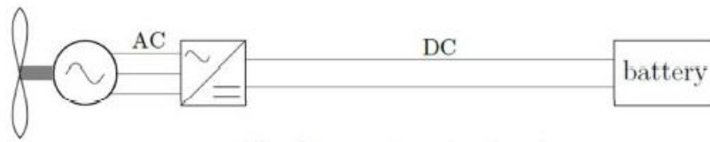
Figure 2.1: "Configuration Diagram Full Electric" - System Analysis of Turbo-Electric and Hybrid Electric Pro-pulsion Systems on a Regional Aircraft – 2018
