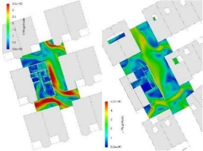
Figure 35 Ventilation simulation on the 5m elevation plane of No. 3 and No. 4 sample dwelling houses under the prevailing wind Source: Self-painted
