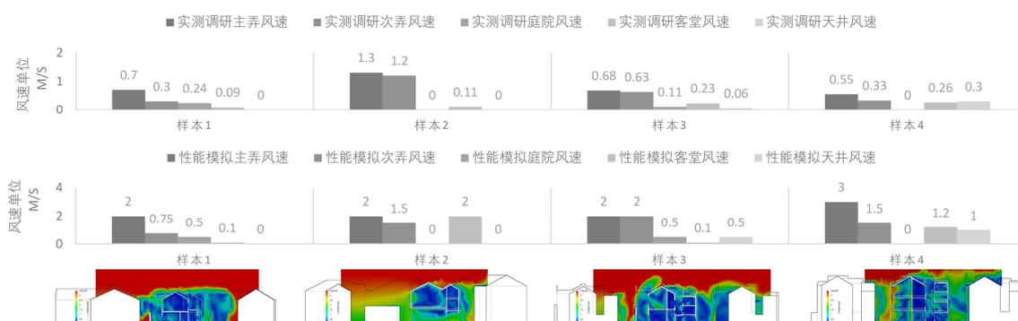
Figure 41 Interactive verification of field measurement of wind speed gradient and performance simulation Source: Self-drawing
