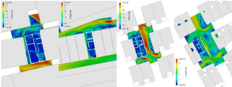
Figure 34 The plane ventilation simulation of four sample dwellings at an elevation of 1.7m under the prevailing wind Source: self-painted
