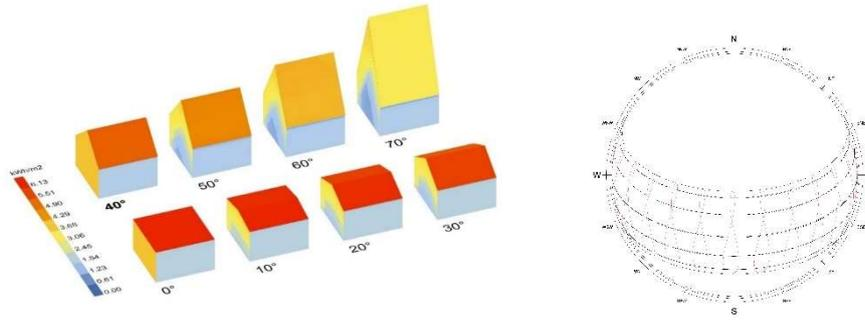
Figure 28 (Left) Relationship between roof thermal inclination angle and solar radiation in Shanghai area Source: Self-painted
