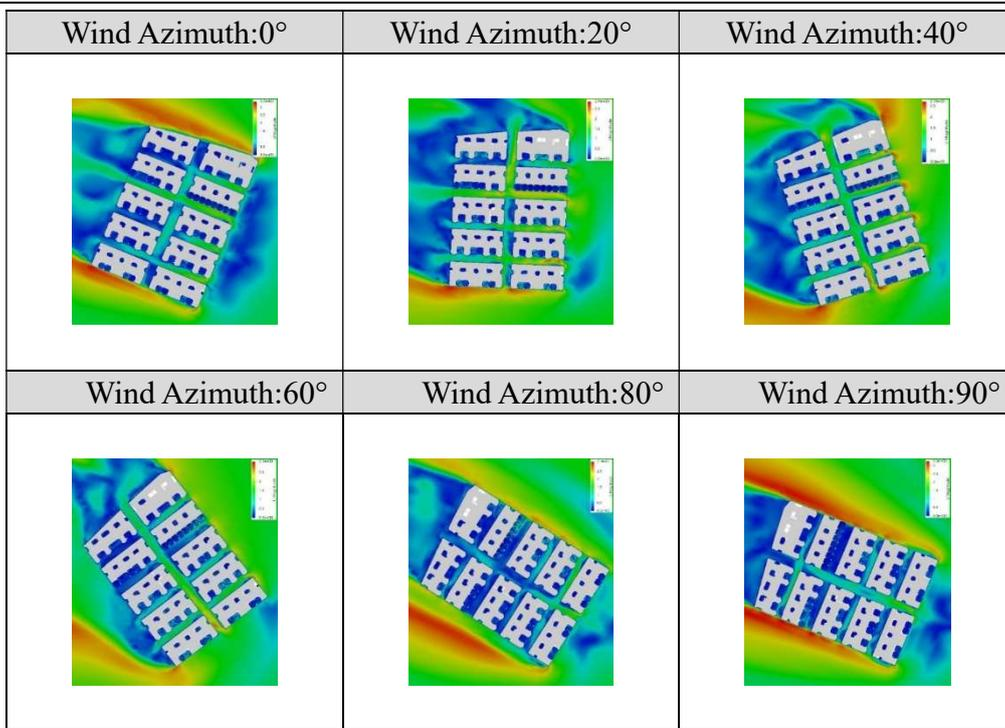
Table 12 Simulation of wind pressure at different wind azimuth angles in Siming Village
