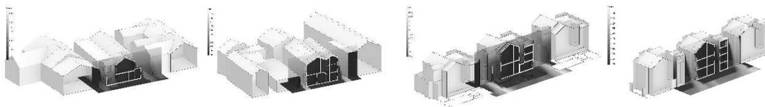
Figure 55 The shadow density indication of sample with void body aspect ratio 2.4, 2.8, 1.8, 2.1 Source: self-painted
