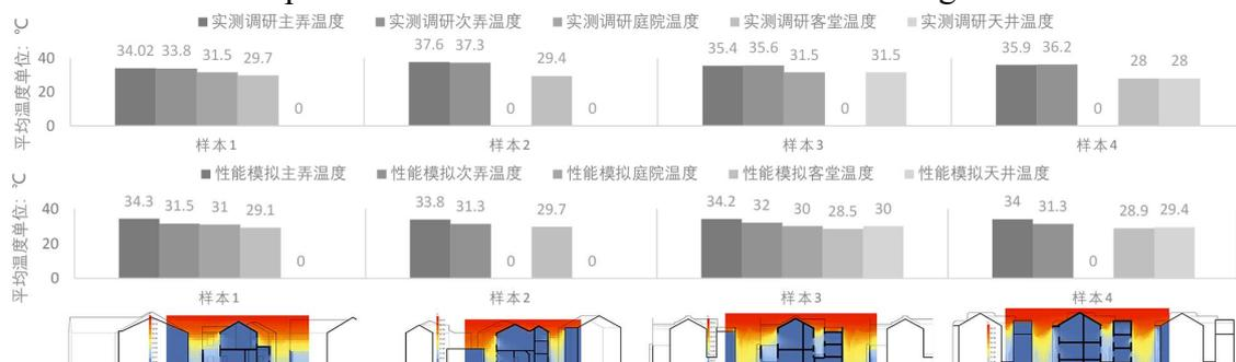
Figure 42 Interactive verification of field measurement of thermal gradient and performance simulation Source: Self-drawing
