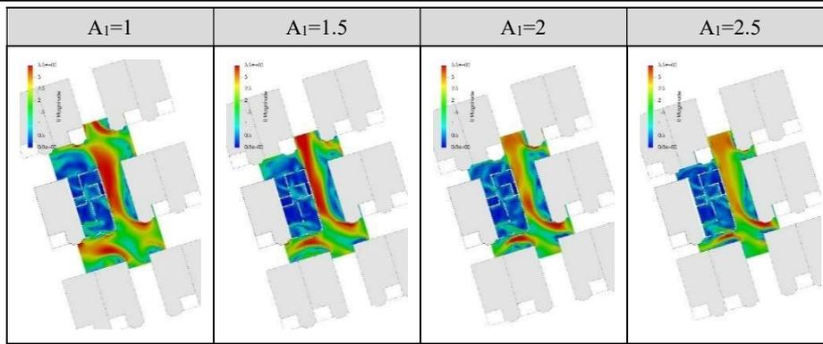
Table 25 Wind Environment Simulation of Sample 3 with Different Courtyard Aspect Ratio
