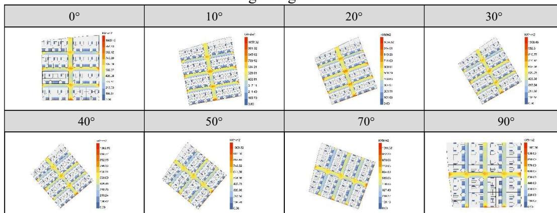
Table 16 Sun radiation simulation of buildings with different thermal azimuths in Siming
