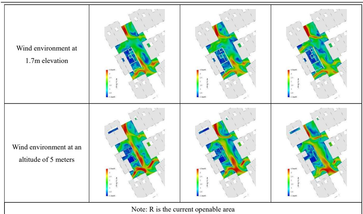
Table 45 The north-south openable area ratio variable and thermal environment simulation
