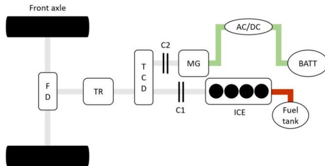
*Figure 10. Powertrain configuration of parallel P2-HEV (case study)*
