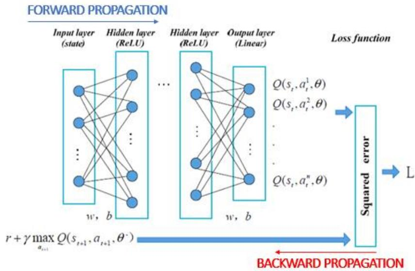
Figure 17. Structure of the neural network
