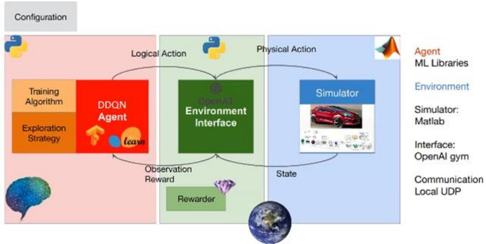
Figura 24. Software framework configuration
