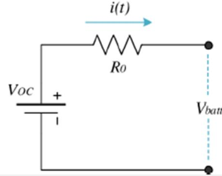
Figure 13. Internal resistance model of the battery (Rint model)
