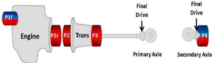
Figure 7. P-method for simple parallel-HEV
