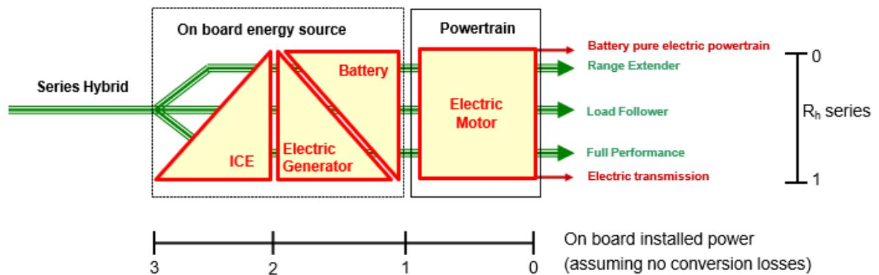
Figure 3. Simple Thermal-Electric series-HEV
