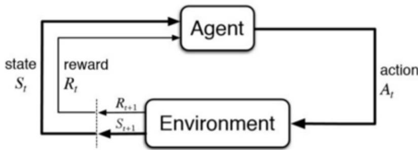
Figure 15. Basic concept of Reinforcement Learning
