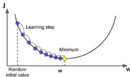
Figure 20. Gradient descent (cost function as function of weights)
