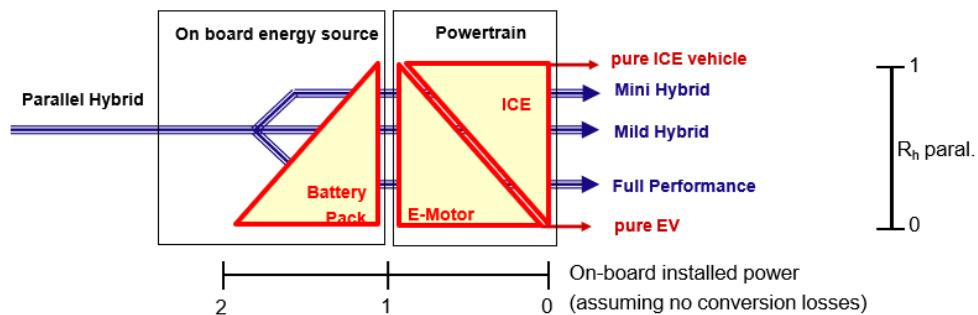
Figure 4. Simple Thermal-electric parallel-HEV
