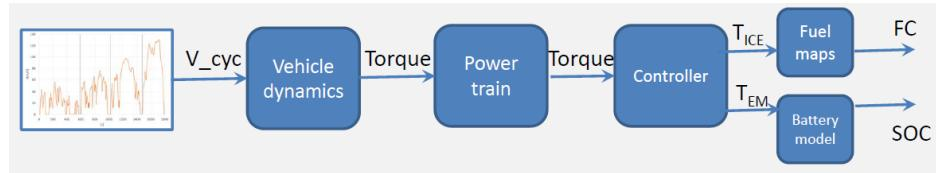
Figure 12. Kinematic vehicle simulator (quasi-static simulation)
