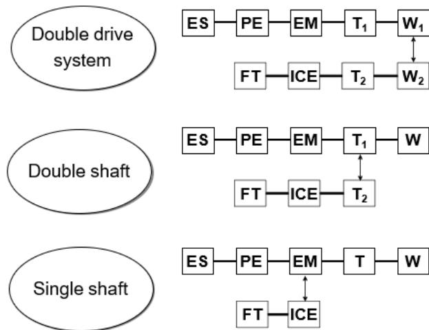
*Figure 5. Classification of simple parallel-HEV (Beretta method)*
