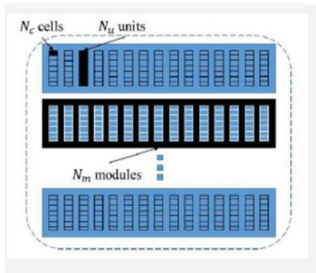
*Figure 14. Typical architecture of high voltage Li-Ion battery*
