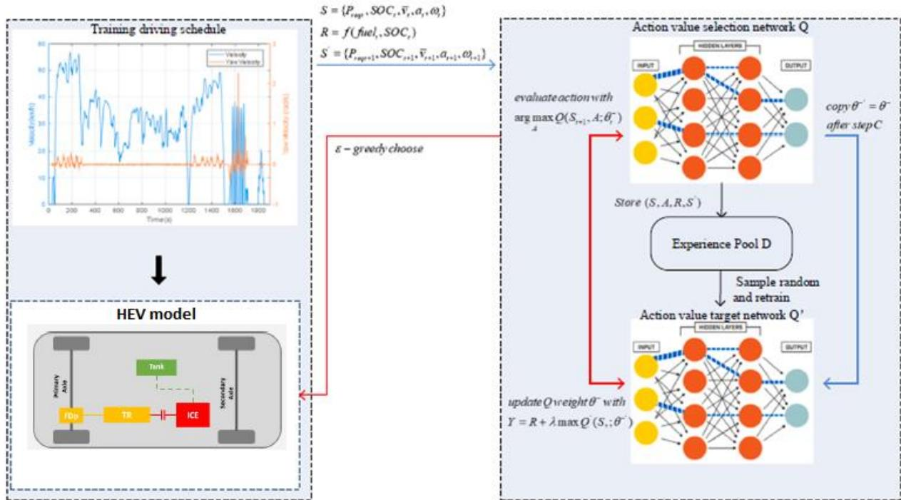
Figure 23. Process of the energy management strategy based on DDQN algorithm
