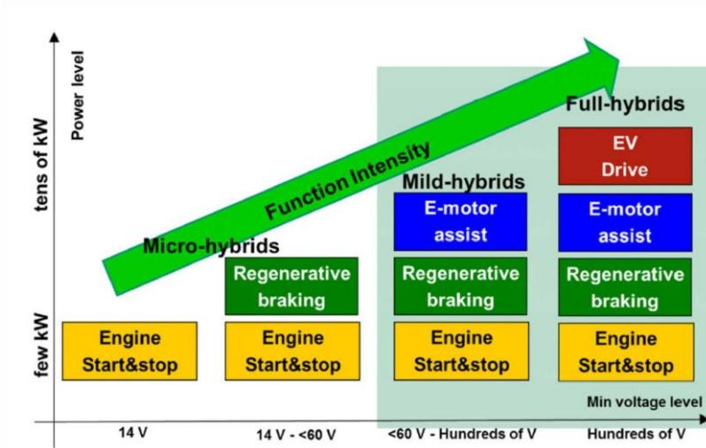
*Figure 2. HEVs classification based on power and voltage*
