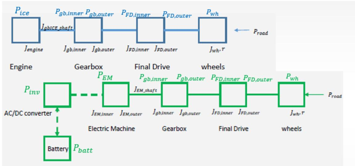
Figure 11. OD-kinematic model for ICE (up) and EM (down)
