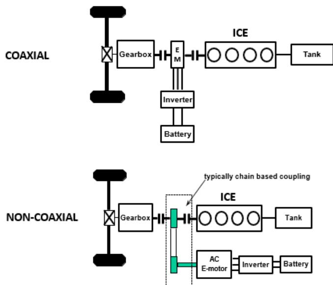
Figure 6. Single shaft: Coaxial and non-coaxial solution
