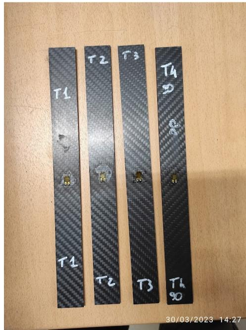
*Figure 4.3: Tensile Specimen-before the test*
