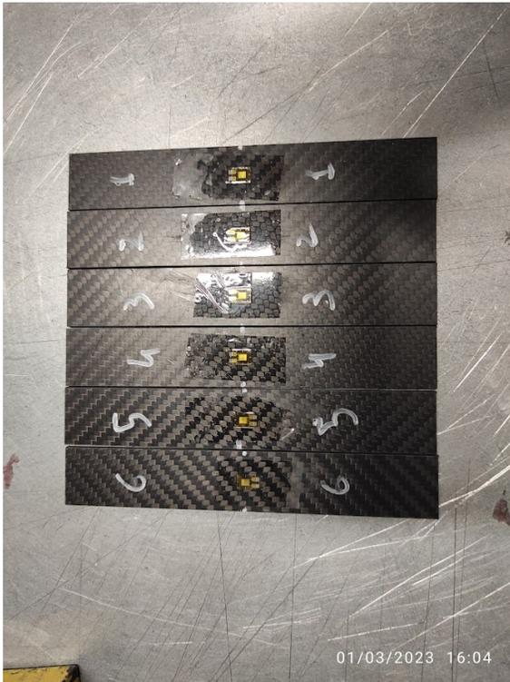
(a) Specimen with strain gauges applied
