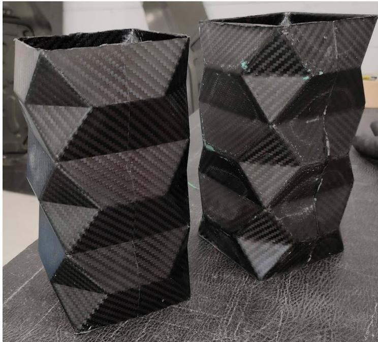
*Figure 5.12: Impact validation specimen*
