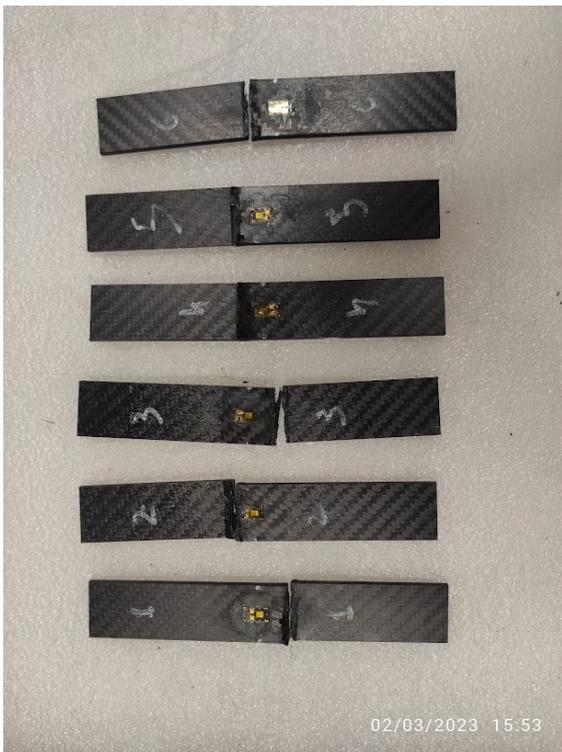
(c) Compression specimen-after the test
