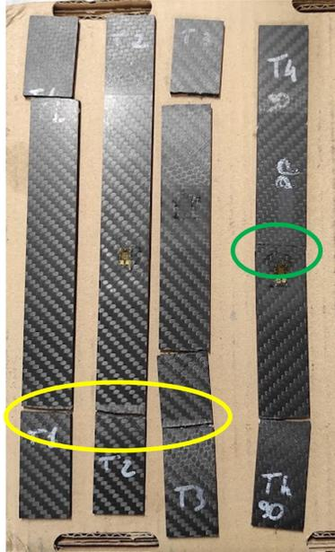
Figure 4.4: Tensile Specimen – after the test
