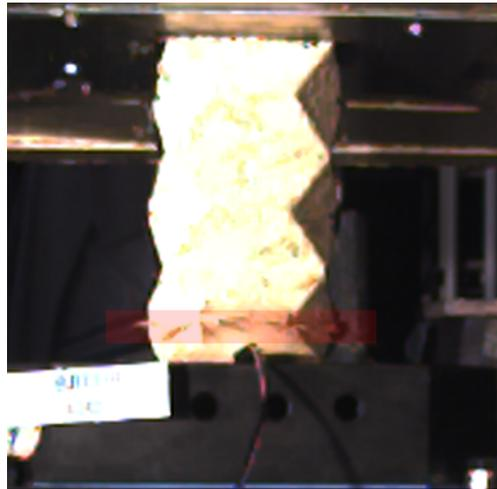
Figure 7.2: First failure point - crash box
