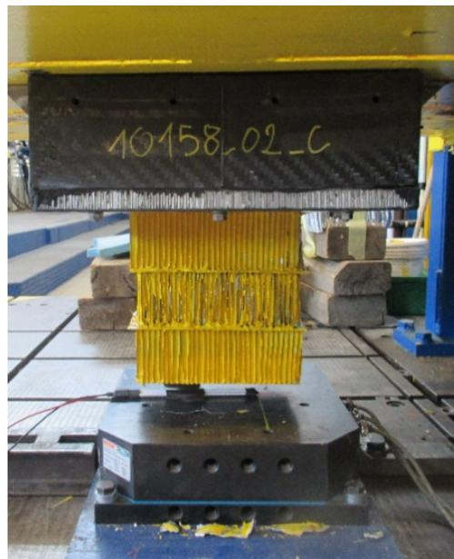
*Figure 8.3: Previous attenuator structure*
