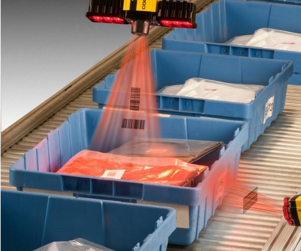
*Figura 4.5: fixed mount reader. Fonte: <https://www.ssetechnologies.com/fixed-mount-barcode-scanner-blog/>*
