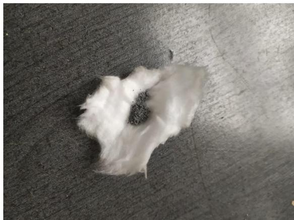
Figure 49. Sample of aluminium in the quartz wool for tube-in-tube reactor testing.
