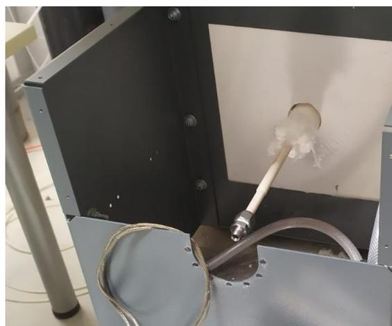
Figure 46. Tube-in-tube reactor – output section.
