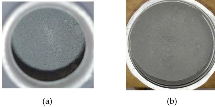
Figure 68. Appearance of the coarse powder (a) and fine powder (b).
