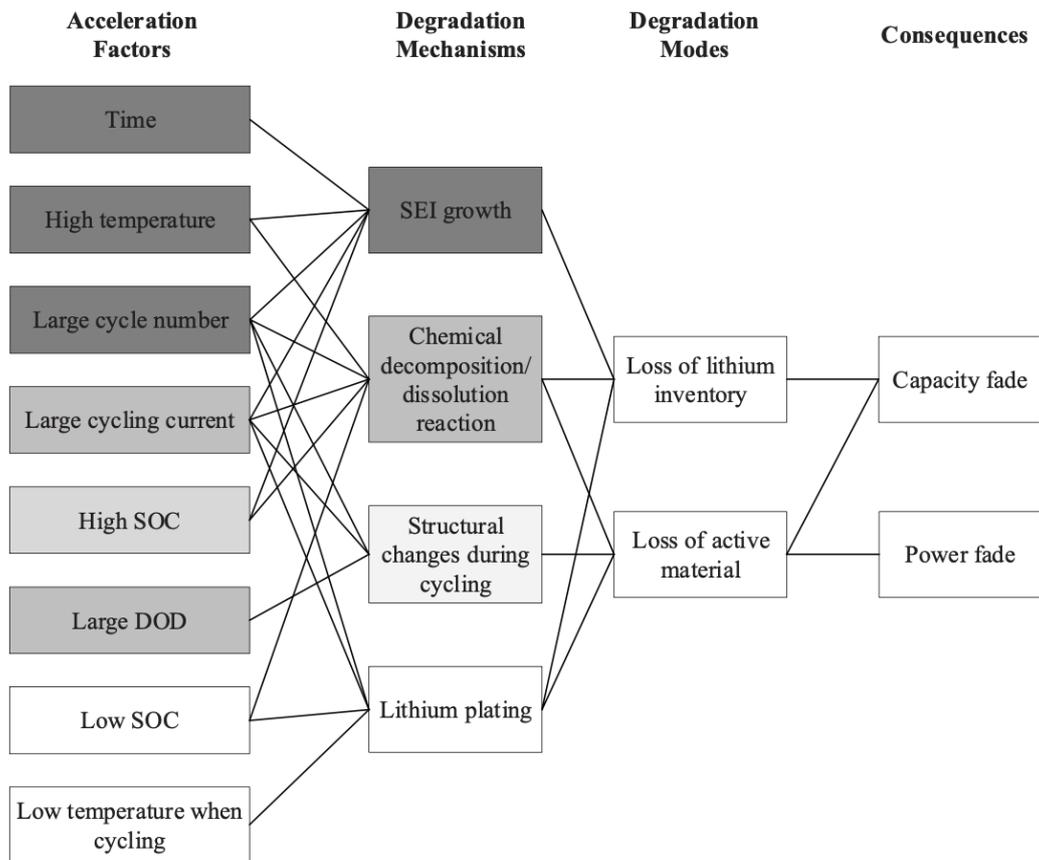
Figure 1: Battery degradation components [7]
