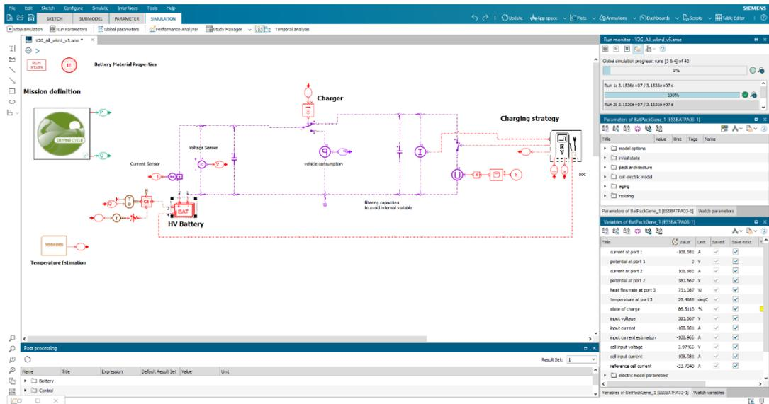
Figure 17: Full model interface & HV battery parameters list
