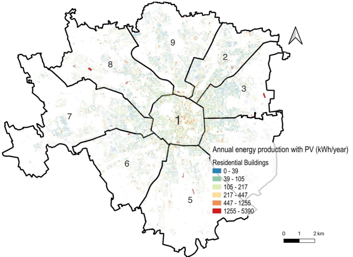
**Figure 21.** Annual energy production with roof-integrated Photovoltaic panels.
