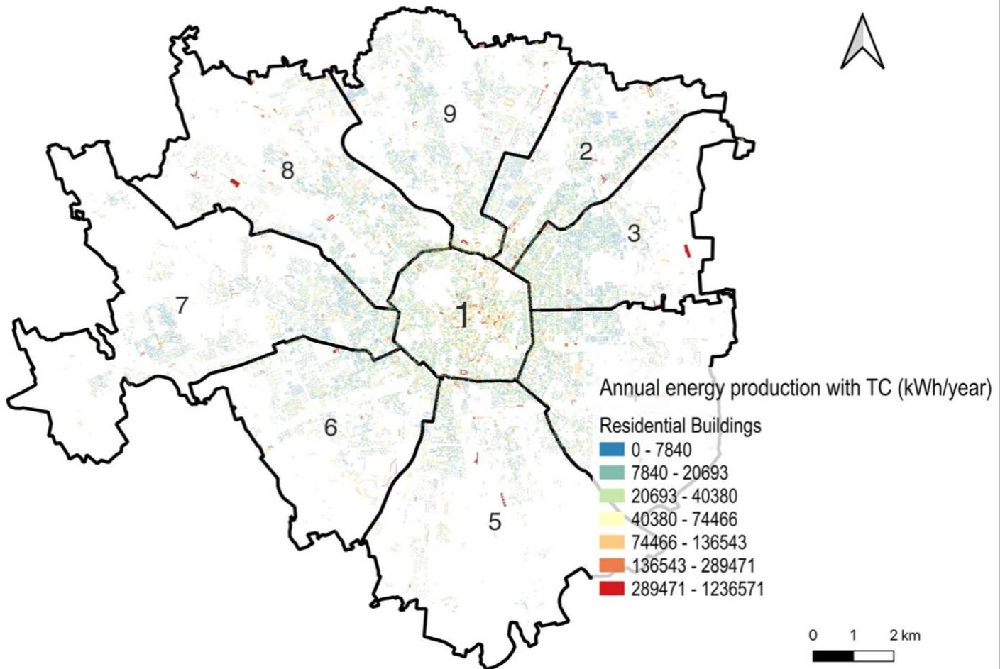
**Figure 22.** Annual energy production with roof-integrated solar thermal collectors.
