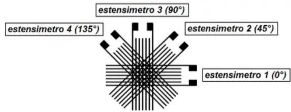
**Figure 2.9 Doorstopper strain gauges**
