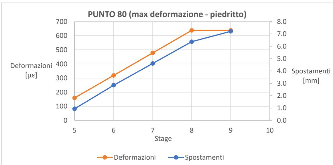
**Figure 3.14 maximum strain and associated displacement**
