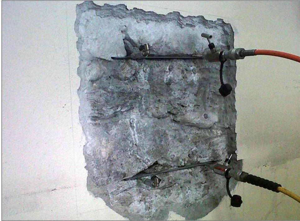
**Figure 2.11 Flat-jack test ([www.sisgeo.it](http://www.sisgeo.it))**
