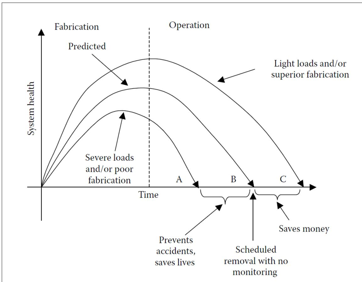
**Figure 1.1 Potential utility of system and SHM versus operation without monitoring (Huston, 2010)**
