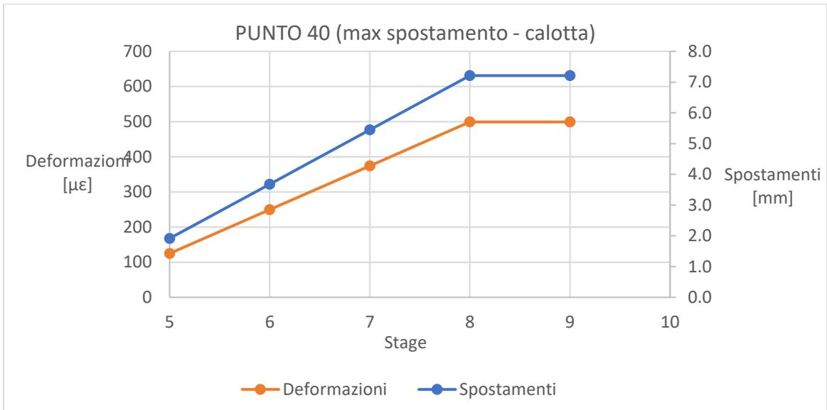
**Figure 3.13 maximum displacement and associated strain**
