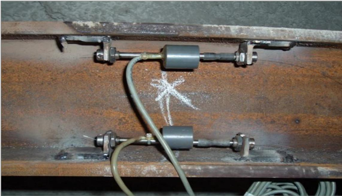
**Figure 2.2 vibrating wire gauges bolted to the rib. (Bilotta & Russo, 2016)**
