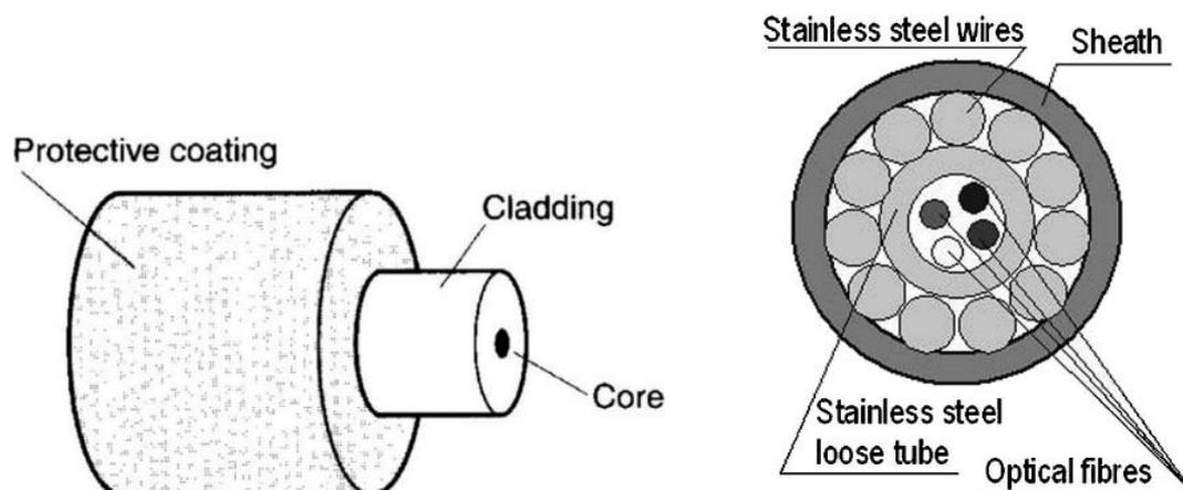
**Figure 1.6 Fiber optic wire (Das & Saha, 2018)**
