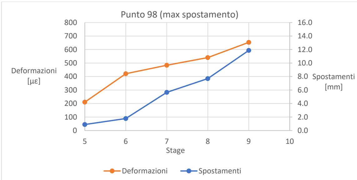
**Figure 3.21 maximum displacement and associated strain**
