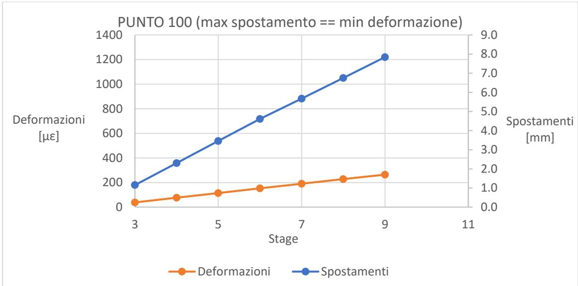
**Figure 3.16 maximum displacement and associated strain**
