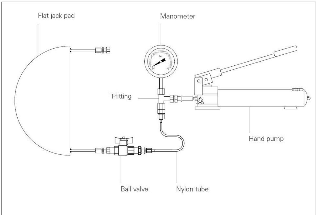
**Figure 2.12 Flat-Jack device ([www.sisgeo.it](http://www.sisgeo.it))**
