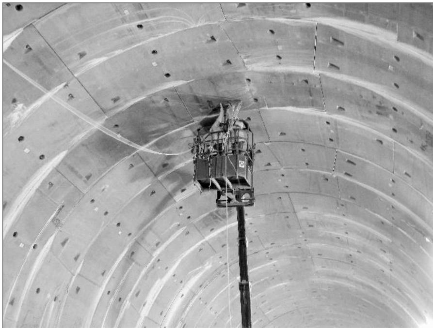
**Figure 2.10 Doorstopper application in tunnel lining (Guido et al., 2021)**
