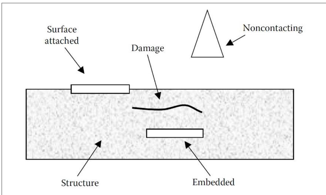
**Figure 1.3 Sensor location relative to structures (Huston, 2010)**
