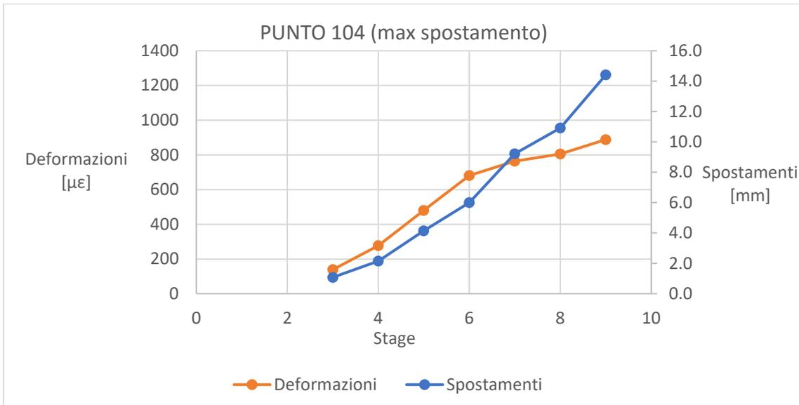
**Figure 3.19 maximum displacement and associated strain**
