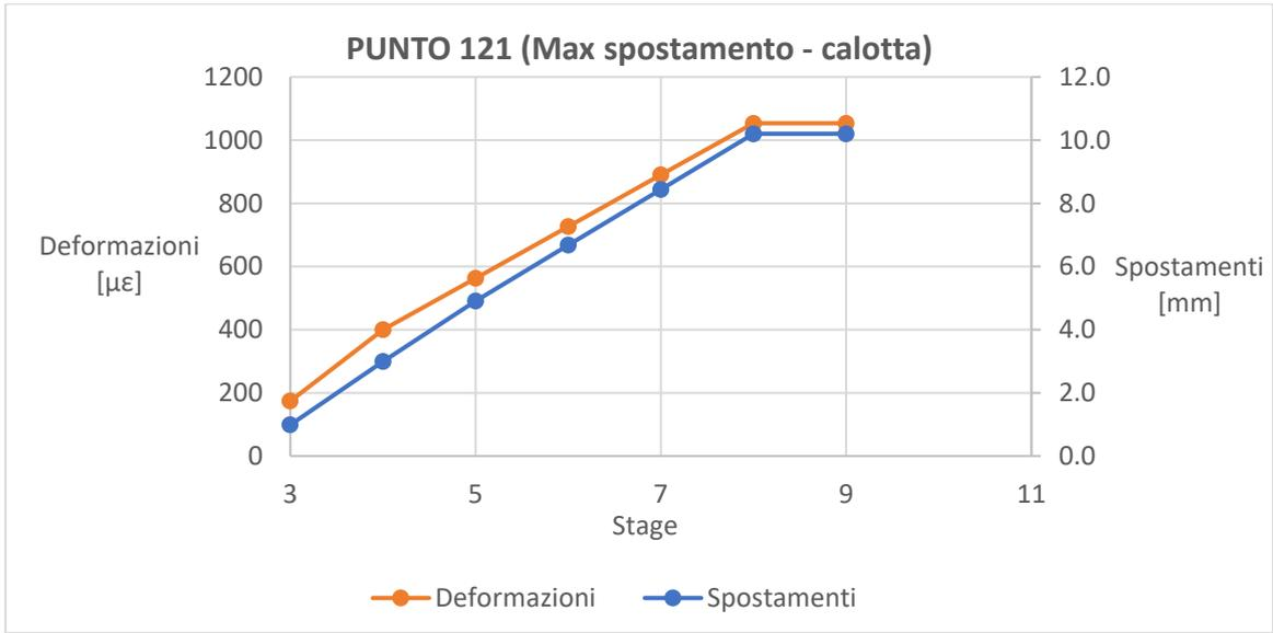
Figure 3.11 maximum displacement and associated strain
