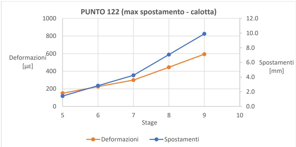
**Figure 3.8 maximum displacement and associated strain**
