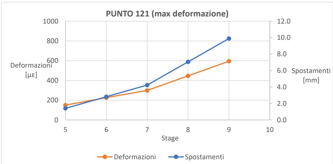
**Figure 3.9 maximum strain and associated displacement**
