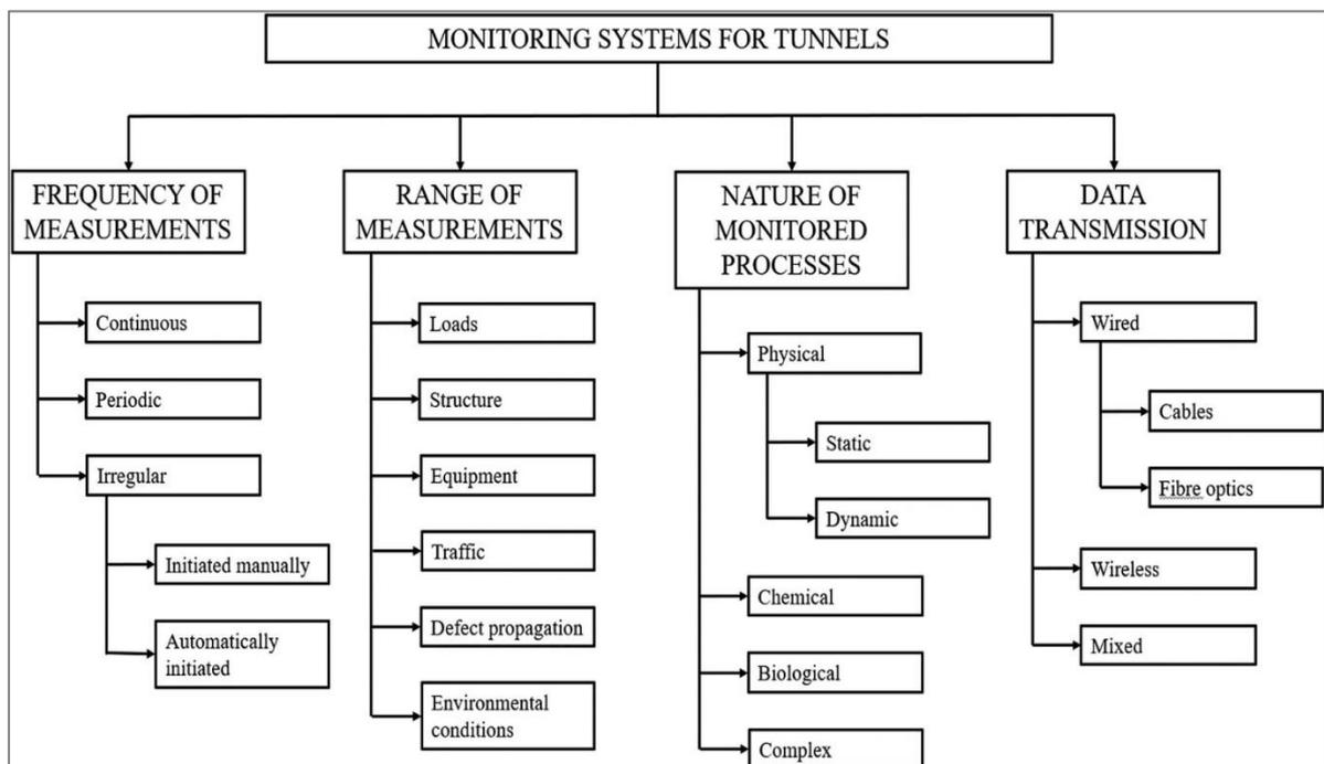
**Figure 2.1 Basic parameters of monitoring system for tunnels (Strauss et al., 2020a)**
