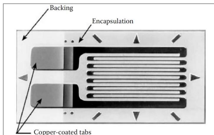
**Figure 1.4 Resistive strain gauge (Huston, 2010)**
