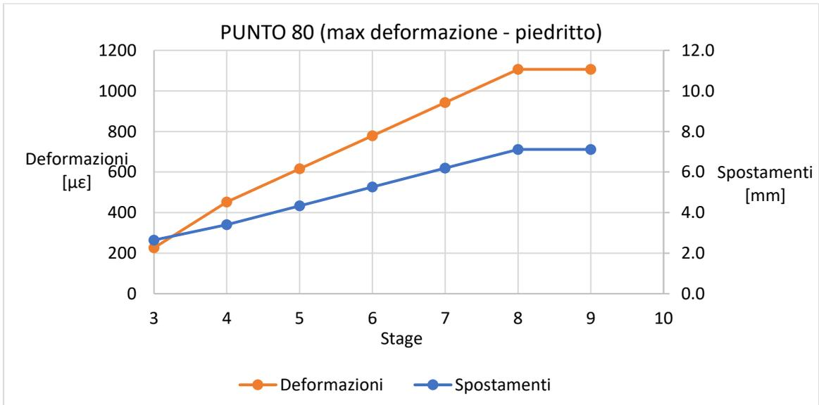
Figure 3.12 maximum strain and associated displacement
