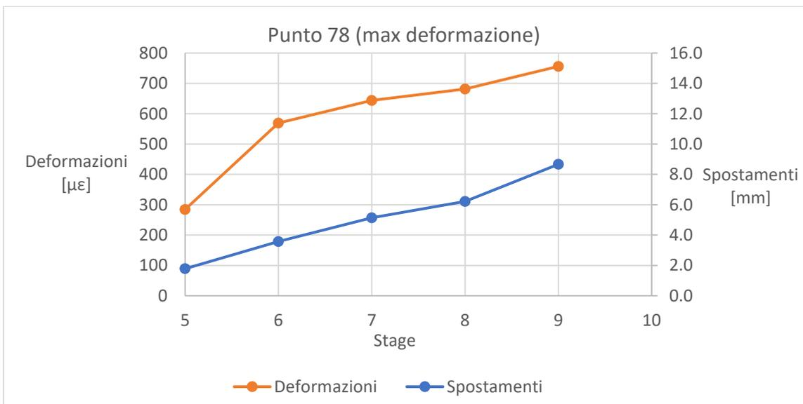
**Figure 3.22 maximum strain and associated displacement**
