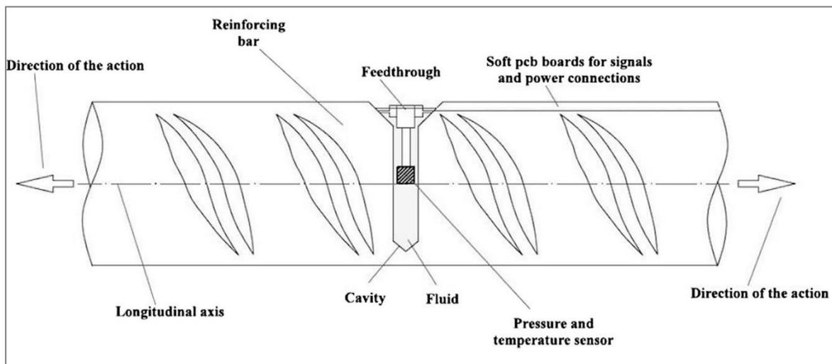
**Figure 1.7 smart steel system (Tondolo et al., 2018)**
