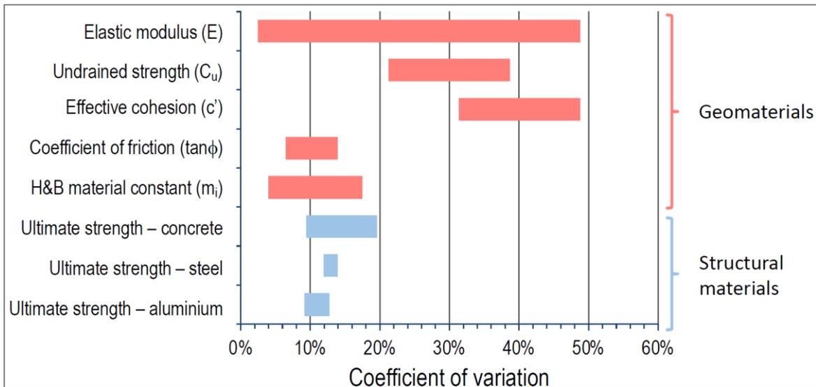
**Figure 1.2 comparison between geotechnical and structural parameters**
