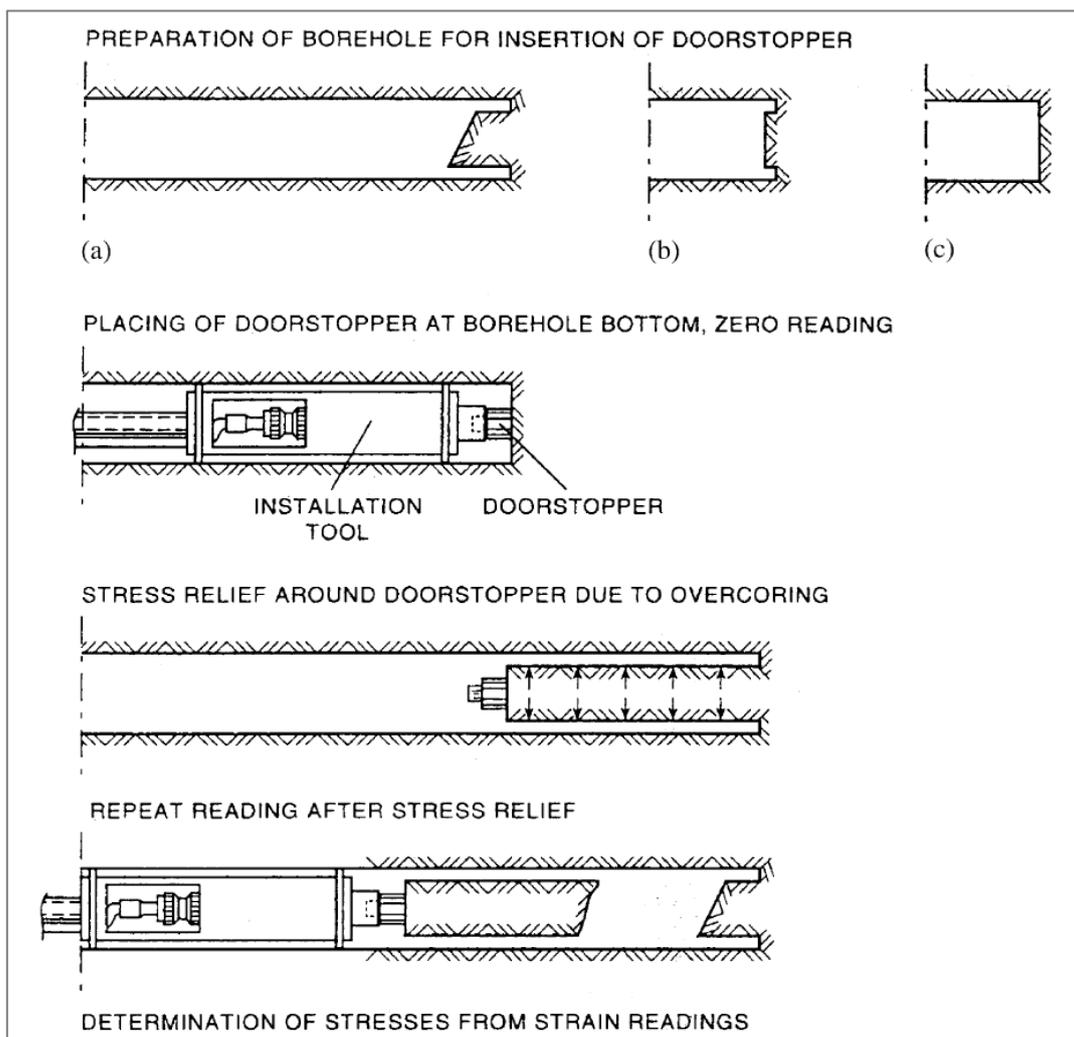
**Figure 2.7 Doorstopper test procedure (Ljunggren et al., 2003)**
