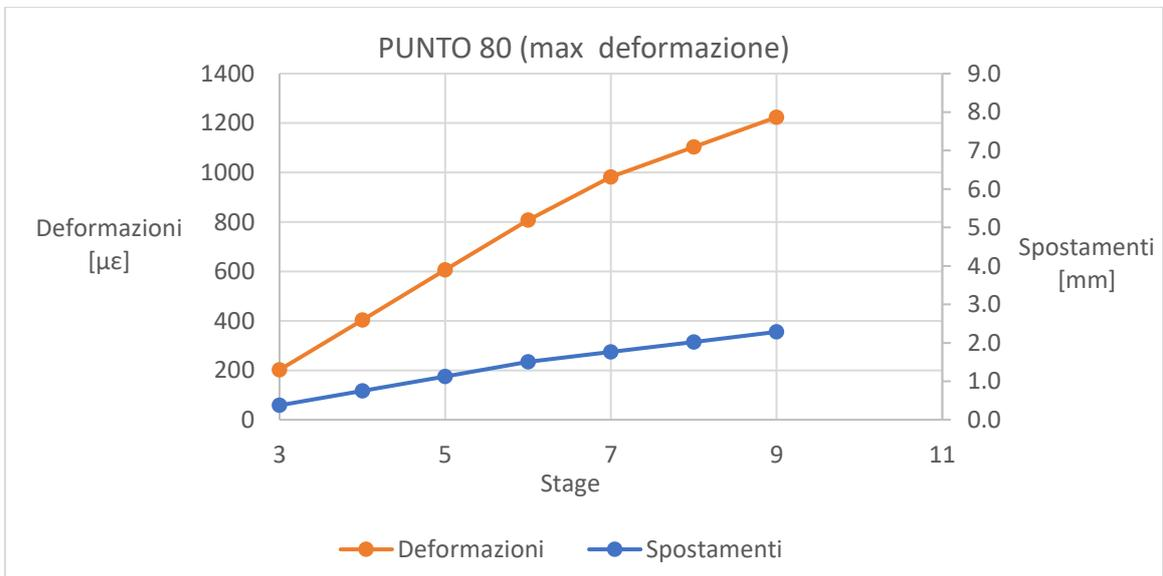
**Figure 3.17 maximum strain and associated displacement**
