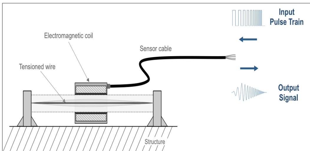
**Figure 1.5 vibrating wire strain gauge (ni.com)**
