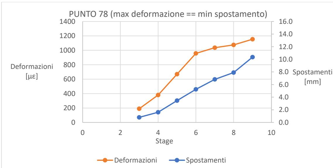
**Figure 3.20 maximum strain and associated displacement**
