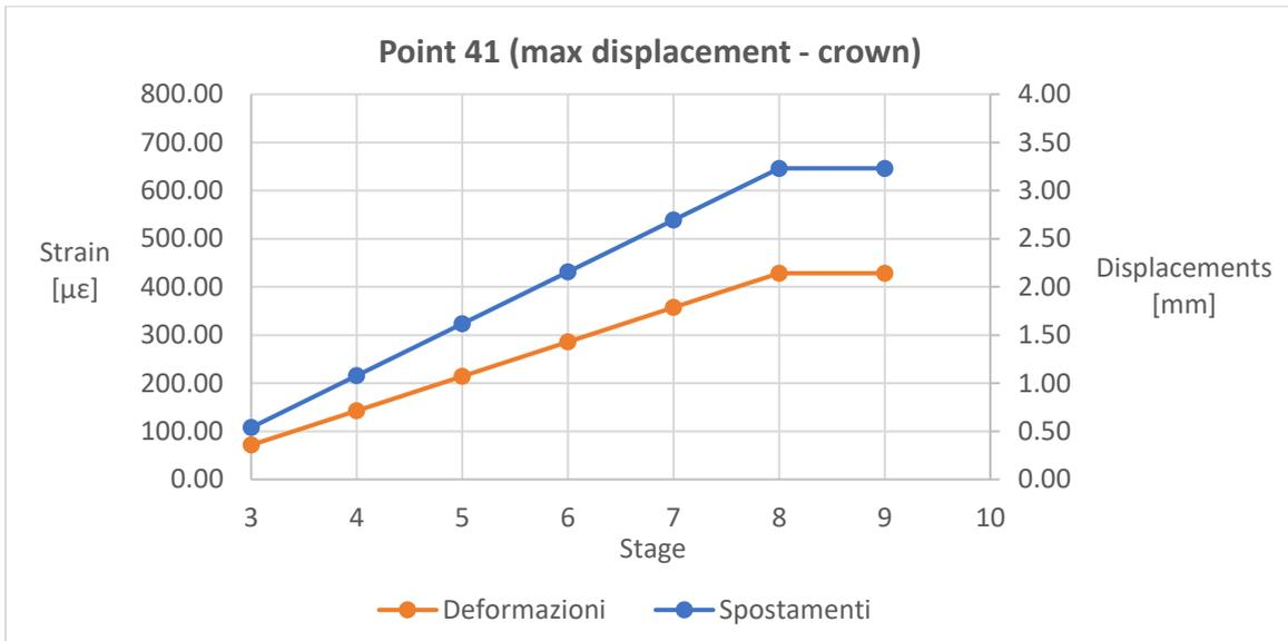
**Figure 3.3 maximum displacement and associated strain**
