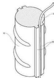
**Figure 1.8 Soft PCB hosted in the bar lug (Tondolo et al., 2018)**
