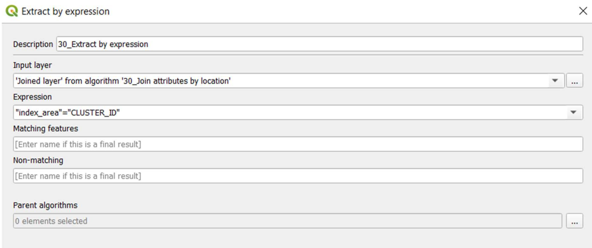
Figure 38 - "Extract by expressions" has been used to extract those points falling inside an isochrone and a buffer area related to the same NLA; " index_area " is the code meaning the belonging to an isochrone (reached domain), " CLUSTER_ID " indicates the belonging to a buffer area (reachable domain).
