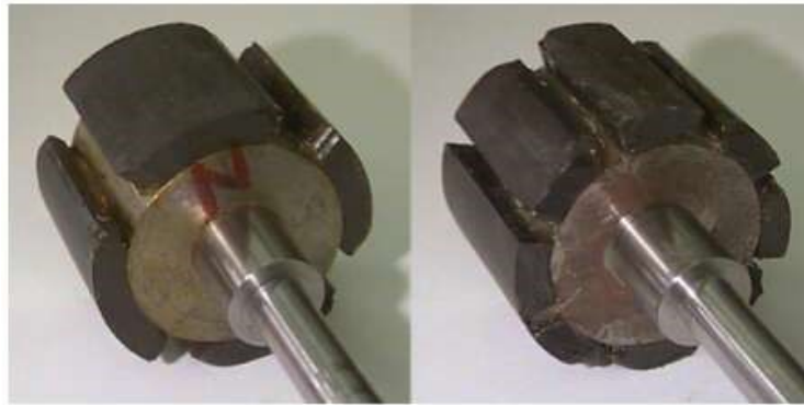
FIGURE 4-14 2 POLE PAIRS ROTOR [LEFT] VS 5 POLE PAIRS [RIGHT]
