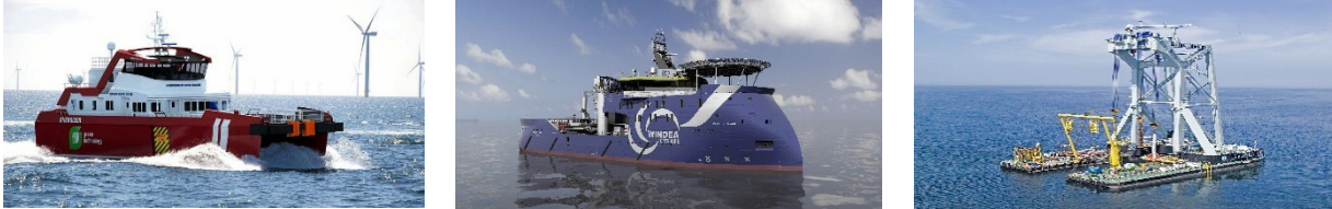
Figure 7. O&M Fleet Vessel Categories: Visual Examples of a) Crew Transfer Vessel (CTV) [39], b) Field Support Vessel (FSV) [40], and c) Heavy Lift Vessel (HLV) [41]
