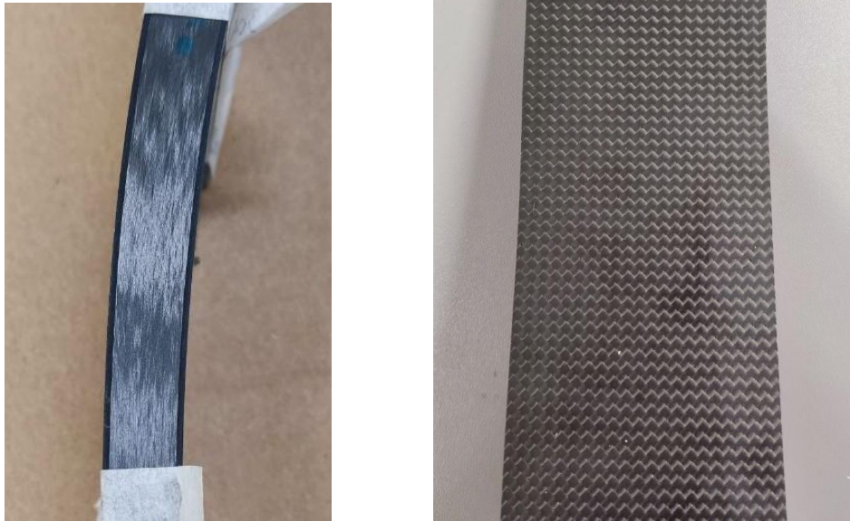
Figure 2.1.6 – Cheetah Xcel Össur material, photos of the frontal (left) and lateral (right) views.
