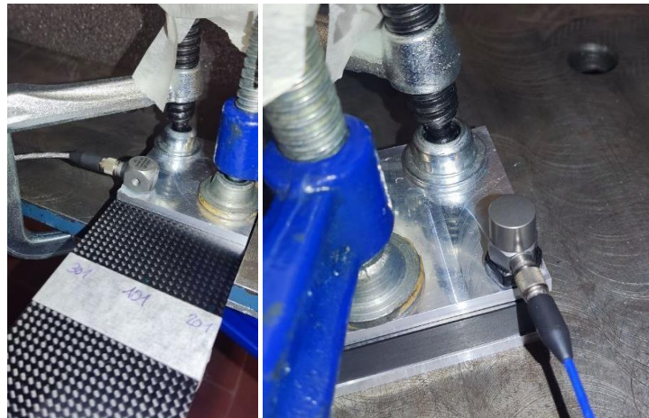
Figure 5.1.1.2 – Details of the implemented hardware, from left to right in reading order: Tri-axial-node 208, Tri-axial-node 305, Tri-axial-node 202, Tri-axial-node 3300, Mono-axial-node 1200.
