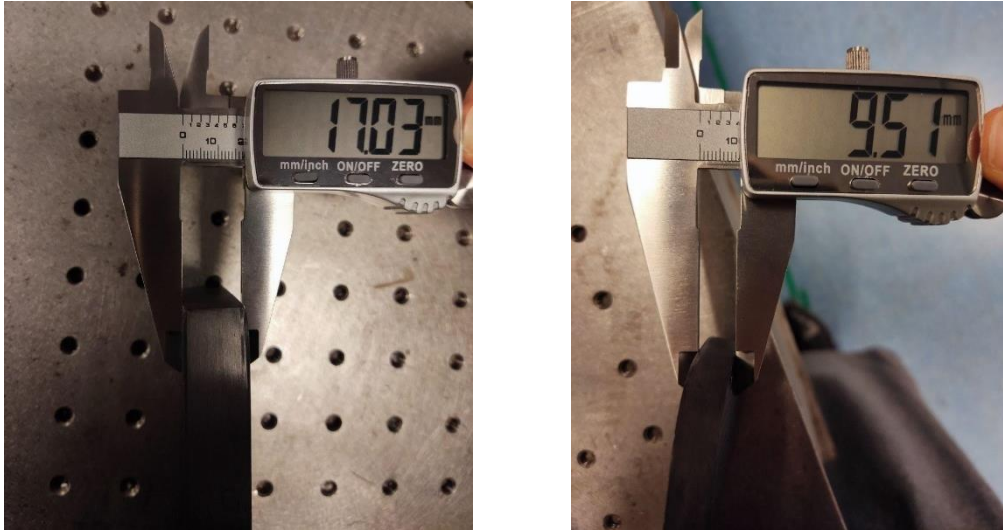
Figure 2.2.6 – Evaluation of the thickness upper (left) and lower (right) ends on the real model through the use of a calibre.
