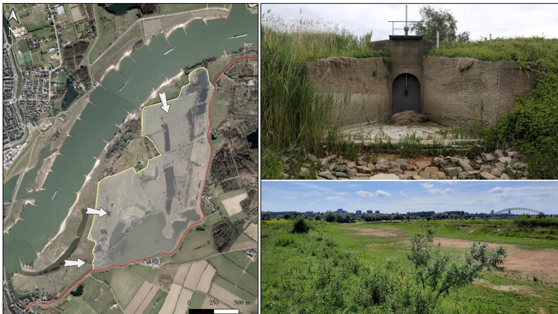
Figure 29. On the left: schematization of the Buiten Ooij floodplain showing the three ways of water entering the storage area depending on the discharge flowing along the Waal. Main dikes (winter dikes) are highlighted by the red line whereas summer dikes are coloured in yellow; Top right: the sluice positioned at the downstream end of the floodplain area (corresponding to the lowest arrow of figure on the left), (source: from Kurstjens et al. (2020)) ; Bottom right: Photo of the floodway shot by the middle overflow dike looking downstream (source: photos shot during the field visit shared by Martinengo, M., and Piovani, P.).
