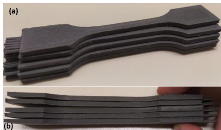
Figure 86. Print result after the planarity calibration: (a) lateral surface view; (b) warping effect due to the thermal shrinkage.
