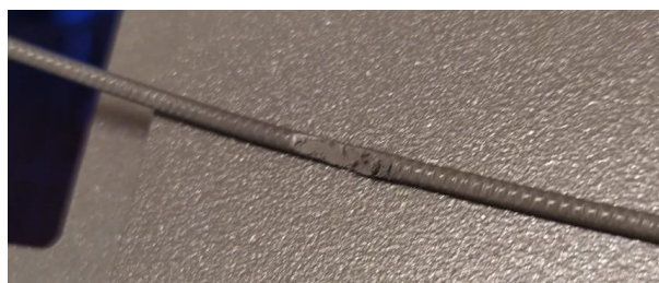
Figure 82. Damage on the filament caused by the feeding system gear.
