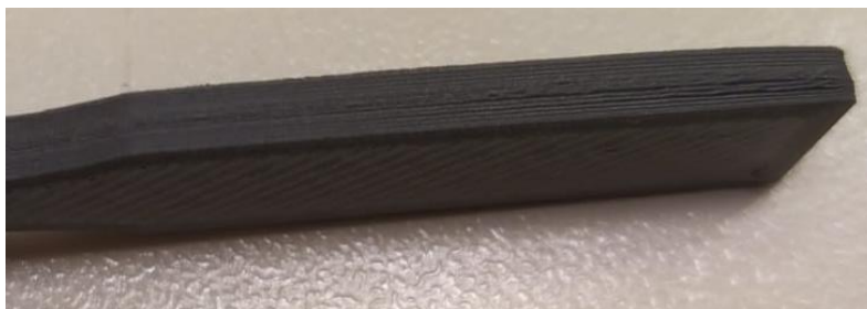
Figure 81. Lateral surface of the fourth trial with visible stripes due to the deadhesion of the first layer.
