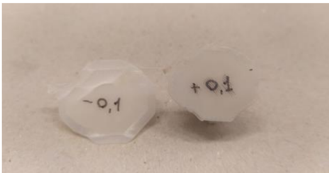
Figure 152. Effect of the gap between the nozzle tip and the bed during the deposition of the first layer.
