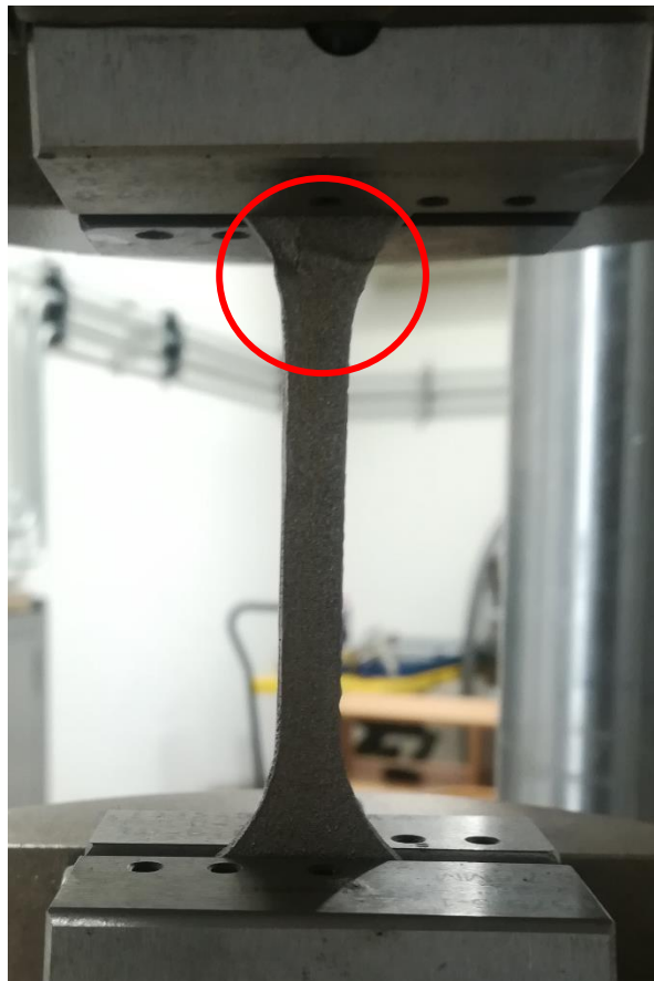
Figure 166. Localization of a defect due to the printing process during the tensile test.
