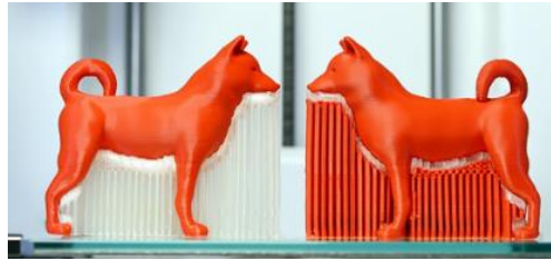
Figure 21. Different way to apply the support material [38].
