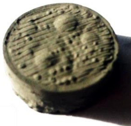
Figure 4. Blistering effect on a specimen with a low pore control [15].
