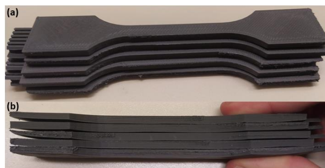
Figure 88. Print result after the removal of the glue from the bed: (a) lateral surface view; (b) warping effect due to the thermal shrinkage.
