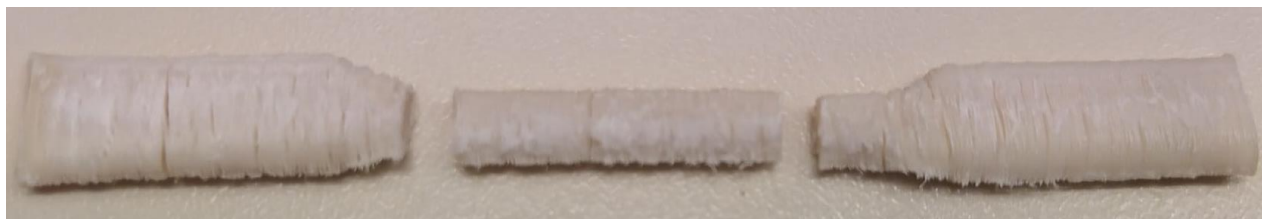
Figure 153. ASA tensile test specimen exposed to the d-limonene for 48 hours.
