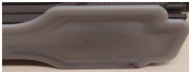
Figure 93. Warping effect of the raft structure due to the thermal shrinkage of the part material.
