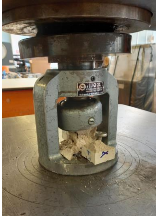
Figure 4. 10: Specimen failed under compressive load
