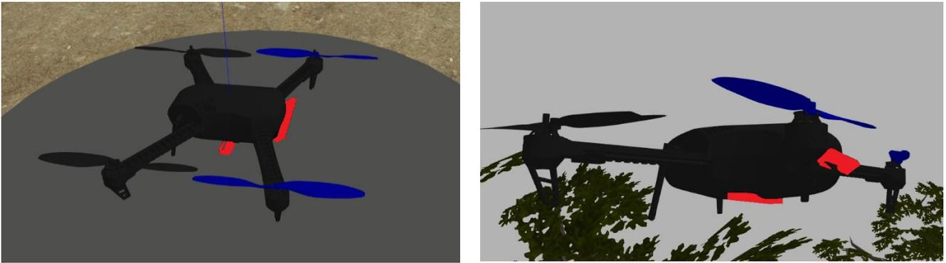
*Figure 2.9: frontal and downward depth cameras highlighted in red fixed respectively on the frontal and lower part of the Iris UAV, as captured in the simulated environment.*
