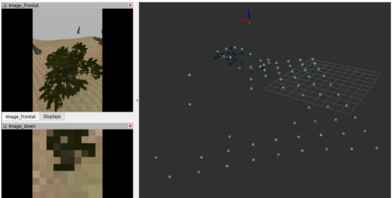
Figure 2.10: Right side: pointcloud generated by the downward camera. Top left: image generated by the frontal camera. Bottom left: Image generated by the downward camera.
