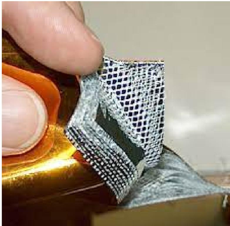
**Figure 2.24:** Close up of Multi Layer Insulation
