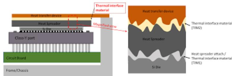
**Figure 2.26:** Function of Thermal Interface Materials
