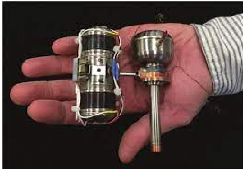
**Figure 2.30:** Micro Cryocooler (Lockheed Martin Space)
