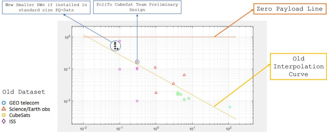
Figure 3.1: Old interpolation Line of reaction Wheels Miniaturization Limit
