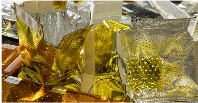
**Figure 2.23:** SoA Multi Layer Insulation (Aerospacefab)
