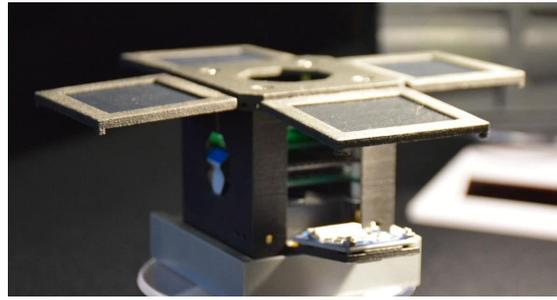
**Figure 2.32:** 3D Printed PQ Satellite (Mini-Cubes)
