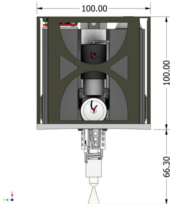
**Figure 2.18:** Green Propellant Micro-Thruster Design from Delft TU
