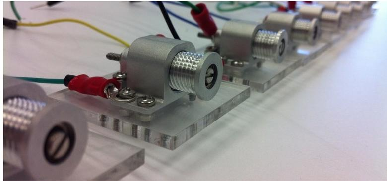
**Figure 2.20:** Miniaturized Concept of a Resistojet Propulsion from the George Washington University
