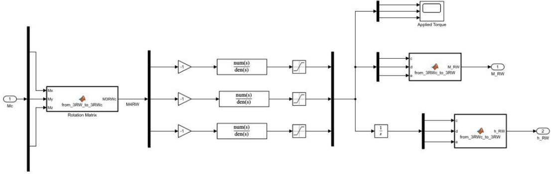
Figure 5.5: Detailed Reaction Wheels Block
