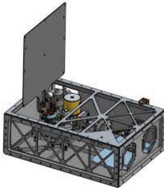
**Figure 2.27:** Example of Deployable Radiator Application in CubeSats (NASA)
