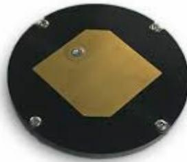
**Figure 2.15:** Miniaturized Omnidirectional Patch Antenna from ISIS Space
