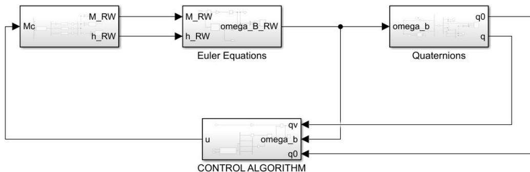
**Figure 5.1:** High Level QFA Block Diagram
