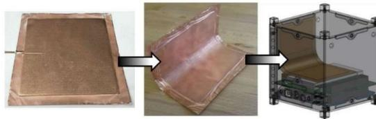
**Figure 2.28:** FlexCool Micro HeatPipe in a 1U frame
