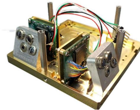
**Figure 2.9:** Miniaturized Horizon Sensor from Adcole Maryland Aerospace
