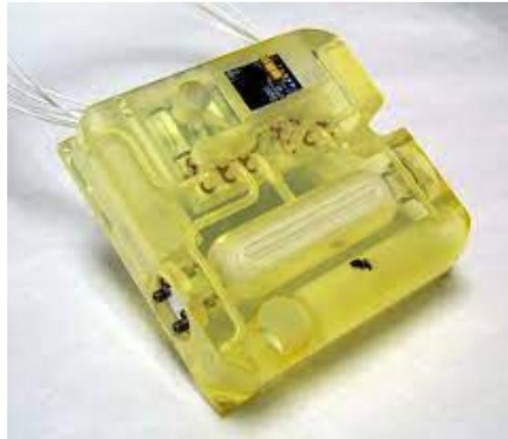
**Figure 2.19:** MEMS Propulsion of the MEPSI Mission
