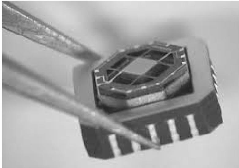
**Figure 2.10:** Chip-Size Atomic Clock (Charles Stark Draper Laboratory)
