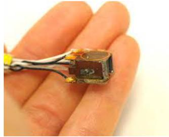
**Figure 2.13:** Miniaturized atomic vapor cell magnetometer (National Institute of Standards and Technology)
