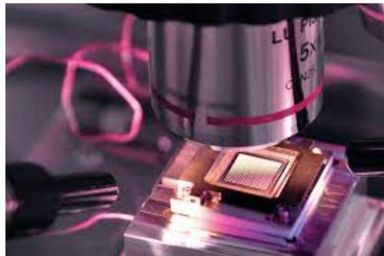
**Figure 2.21:** Miniaturized Concept of ElectroSpray Propulsion from NASA Laboratories
