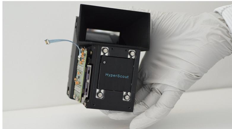
**Figure 2.1:** Hand-sized hyperspectral camera (ESA)
