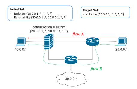
Figure 5.7: Example of deletion of a Reachability requirement
