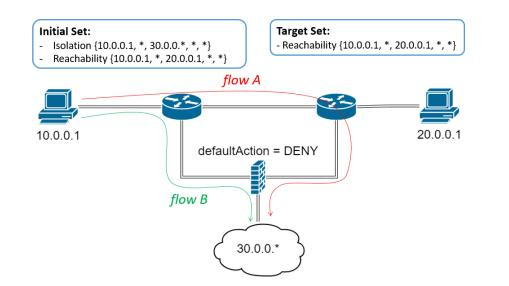
Figure 5.6: Example of deletion of an Isolation requirement
