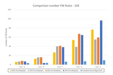
Figure 6.12: Comparison of the number of configured FW Rules for 10X scenario
