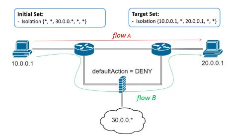
Figure 5.1: Example of addition of an Isolation requirement
