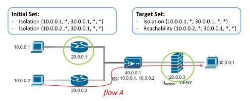
Figure 5.5: Example of special reconfiguration case with new algorithm
