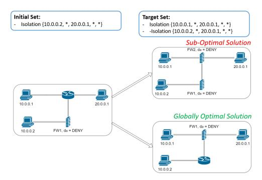
Figure 5.9: Example of the sub-optimality of the proposed reconfiguration approach
