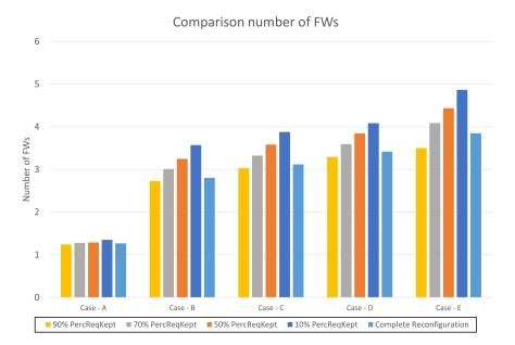
Figure 6.11: Comparison of the number of allocated firewalls
