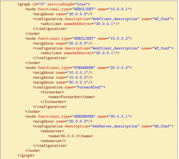
As we see in the listing 3.1, that contains the XML representation of the network in 3.2, each one of the *node* elements represent either a service function or a communication endpoint and it is characterized by different elements:
