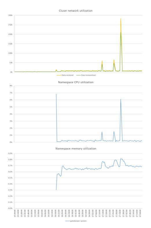
Figure 7.7. Cluster network utilization and resource consumption of the gatekeeper-system namespace.
