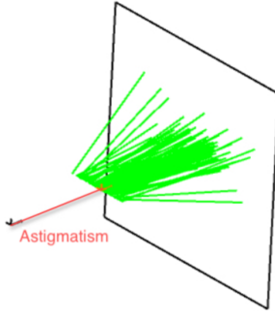
Figure 5.2: Graphical explanation of the Astigmatism parameter from OpticStudio's help guide.
