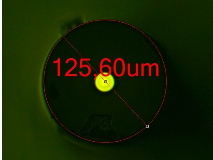
Figure 3.18: BIF cladding diameter measured using microscope.
