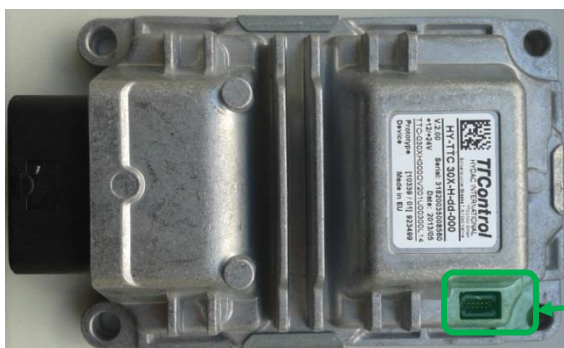
Figure 17: HY-TTC 30 with JTAG connector
