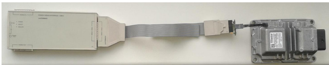
Figure 18: Lauterbach connection to HY-TTC 30X
