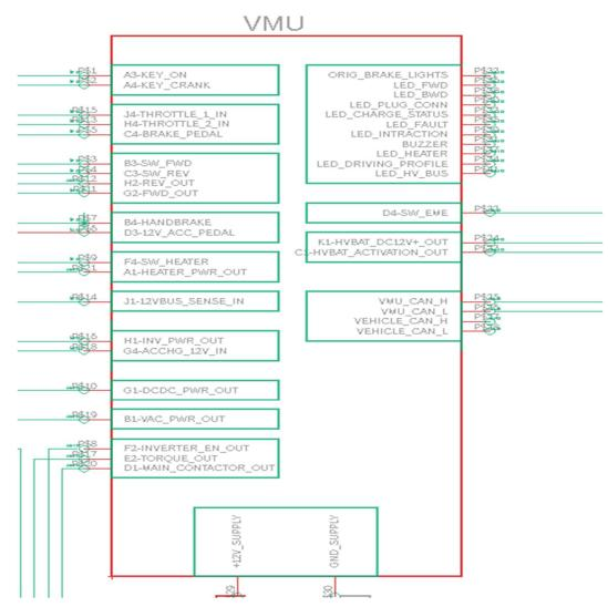
Signal Connector P.N: 571-DRB16-60SAE-L018 and P.N: 571-DRBF-2A used for VMU. The male part of connector will be mounted from inside powerbox.
