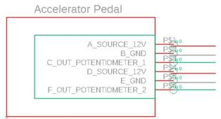
Accelerator Pedal is supplied 12V from a stable voltage source(VMU). There are 6 pins and numbering of pins from top to bottom is done according to workshop manual.
