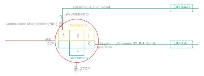
The Key Block (Commutatore di accensione H01) has 5 terminals and 2 connectors i.e Connector A and B. Pin A3 with Signal ID 50 is used for Key Crank( Avviamento) and intermediate connector D004A-G used and Pin B2 with Signal ID INT is used for KEY ON(Marcia) and intermediate connector D001-6 used for it.
