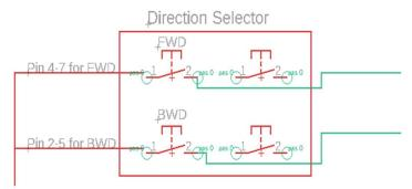
The Direction selector is the Joystick XD2PA24and its detail is available in the <u>Datasheet</u>. It has 4 NO switches. Out of the 8 pins of direction selector, Pin 2-5 NO Switch used for Backward and Pin 4-7 NO switch used for Forward.
