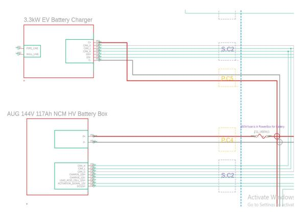
2 pin connector P.N: 829-35254402 fixed on PowerBox and P.N 829-35254366 to connect from other side for High voltage from HV Battery. 450A fuse for battery is inside PowerBox. 3.3kW AC Charger 2 pin connector P.N: 571-2103124-4 fixed on PowerBox. And P.N 571-4-2103177-2 to connect from other side.
