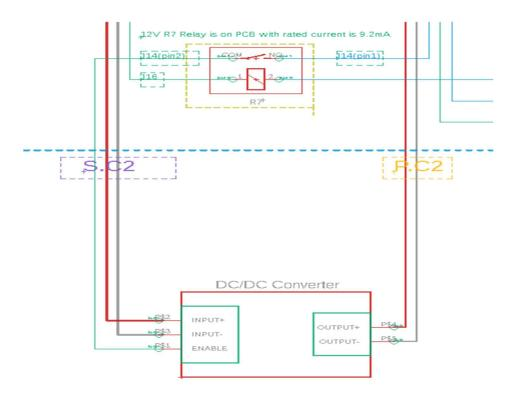
DC/DC Converter is controlled by R7 relay of PCB . J16, J14 connectors used with it. J14, J16 are 2 pins PCB Signal connectors P.N: 87427-0242 fixed on PCB. And P.N: 39-01-2020 to connect from other side. Signal Connector P.N: 571-DRB16-60SAE-L018 and P.N: 571-DRBF-2A used to connect with PowerBox. The male part will be mounted from inside powerbox. DC/DC Converter output connector 2 pin P.N: 571-2103124-4 fixed on PowerBox. And P.N 571-4-2103177-2 to connect from other side.
