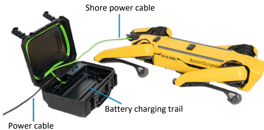
Fig. 15: two ways of charging the Spot battery with other charger models.
