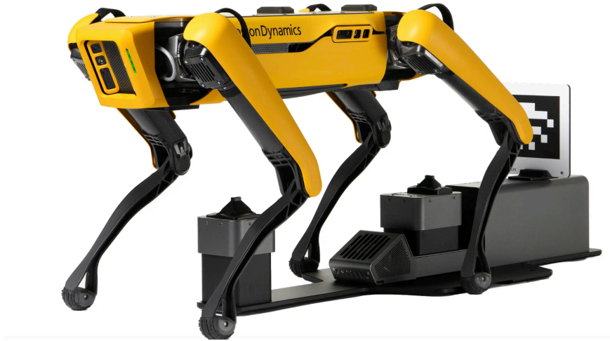
Fig. 16: Spot battery charging exploiting docking station.
