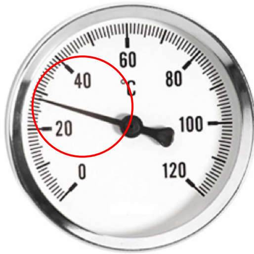
Fig. 35: detection of the pointer in the analog gauge.
