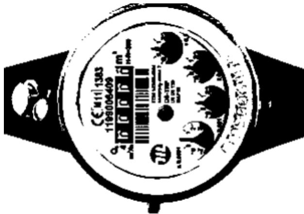
Fig. 31: example of result from the application of a color-based mask on a mechanical water meter.
