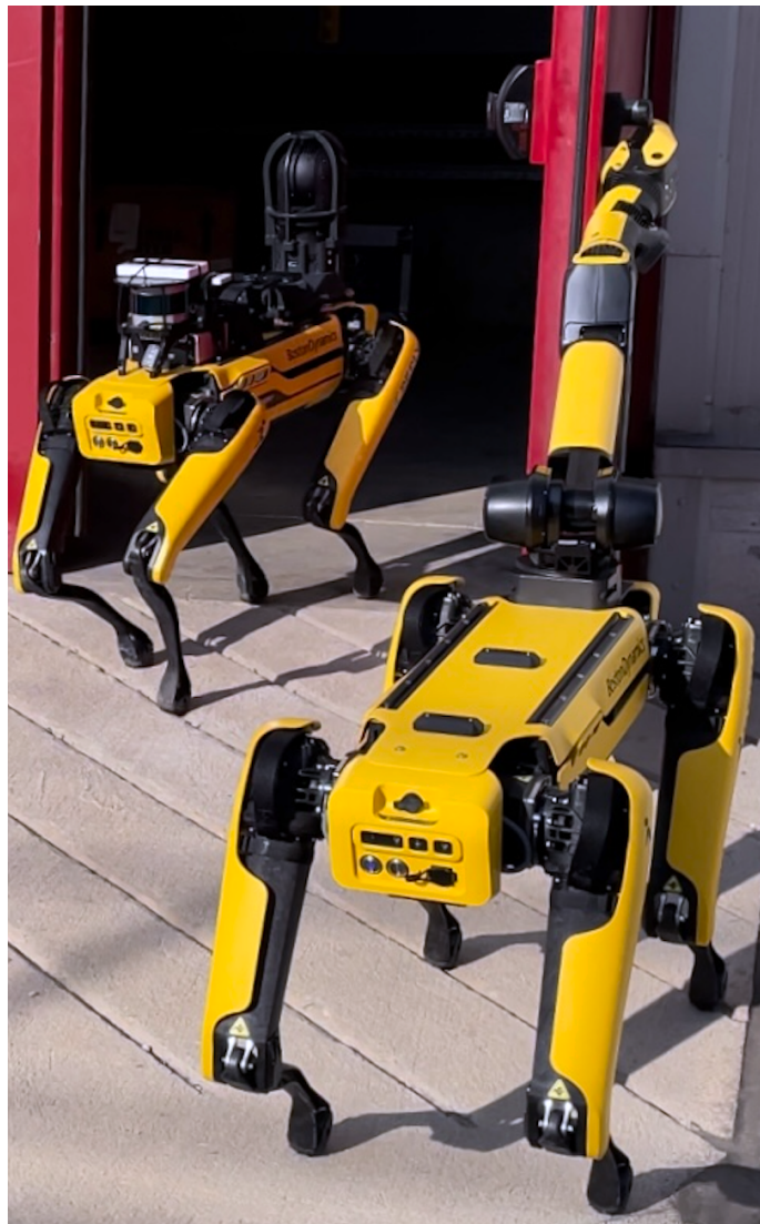
Fig. 56: on-field collaboration between Spot Enterprise and Spot Arm.
