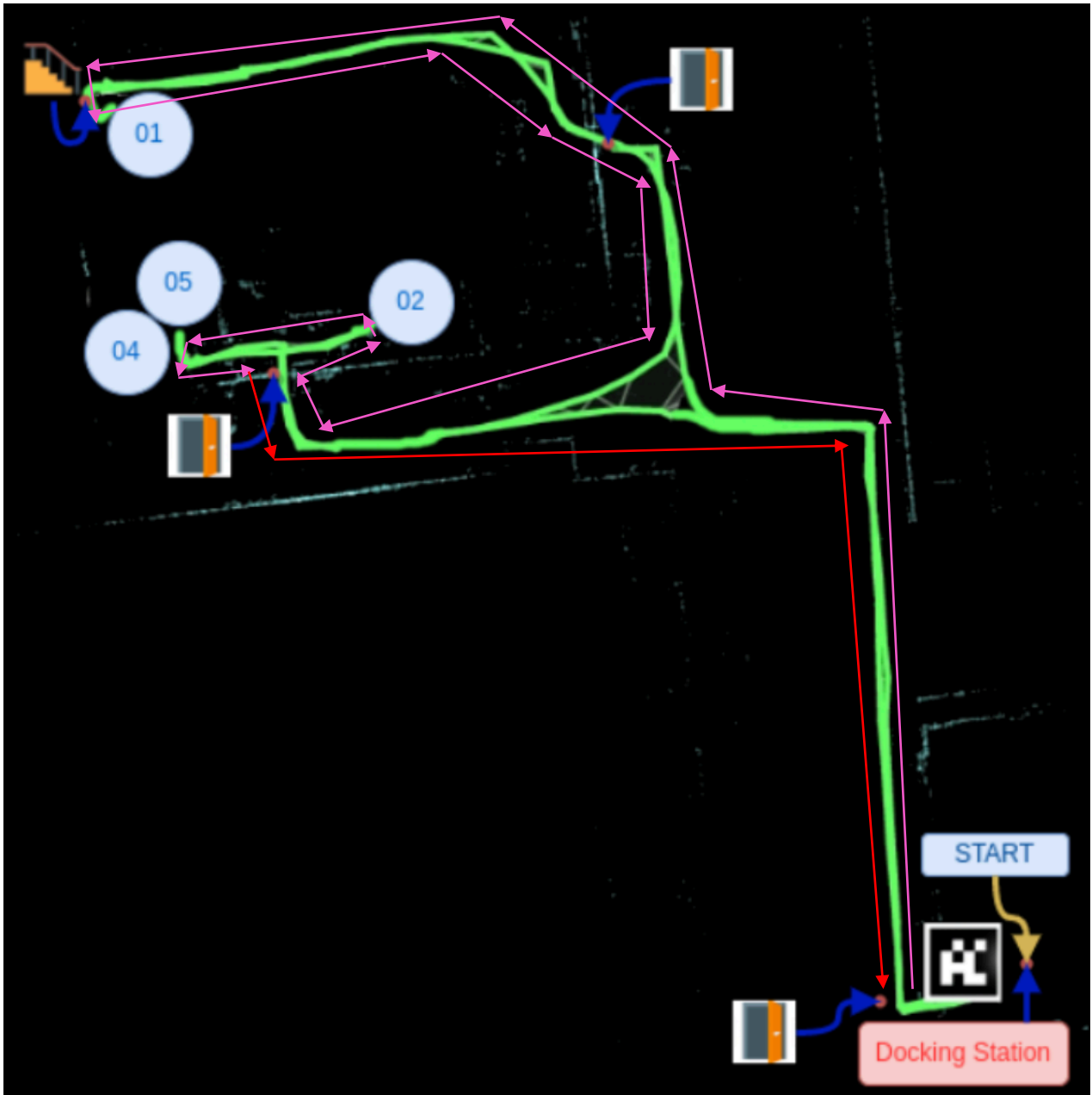
Fig. 47: green solid line identifies the path crossed by Spot in the MISS03 patrol tour; pink arrows depict the direction of the forward path while red arrows depict the direction of the return path.
