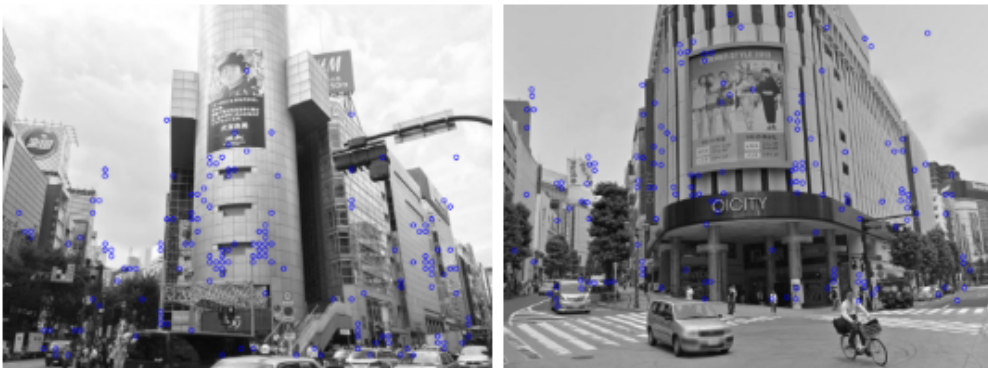
Figure 4.10: LoFTR keypoints . LoFTR is a detector-free model, so we show what points of interest are being considered for matching since it is dependent on image pair.
