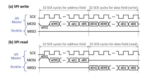
Figure 3.7: 32-bit SPI timing diagram for (a) write and (b) read operations. [9]
