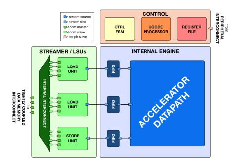
Figure 2.16: Template of a Hardware Processing Engine (HWPE)
