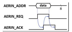
Figure 3.9: Input AER four-phase handshake timing diagram.
