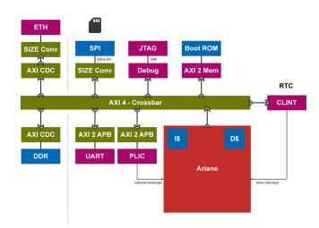
Figure 2.10: Ariane Hardware Control and general purposes Interfaces. [5]
