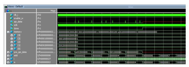
Figure 3.13: wave of security method
