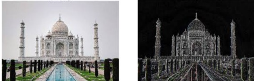
Figure 2.4: Representing the original image before and after Convolution Neural Networks (CNN)[08]
