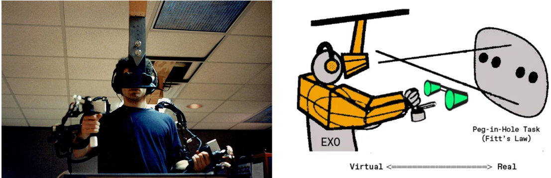
Figure 2.2: “Virtual Fixtures”, the first fully immersive augmented reality system. On the right, a drawing by Louis Rosenberg shows a user of the Virtual Fixtures platform wearing a semi exoskeleton, looking at an actual pin board supplemented by virtual conical fixtures [6].
