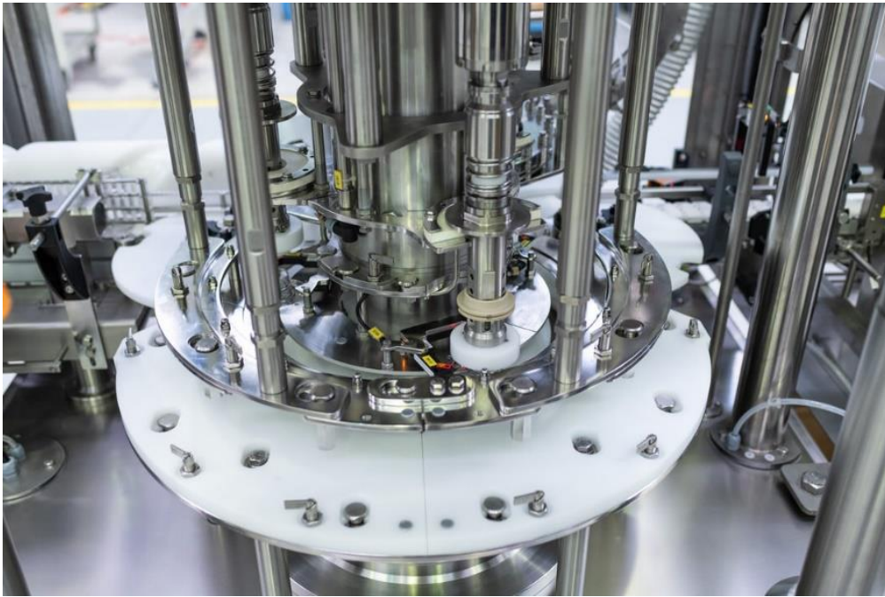
Figure 1.6: Equatorque PK, an example of an AROL capping machinery, close-up view Source: [7]
