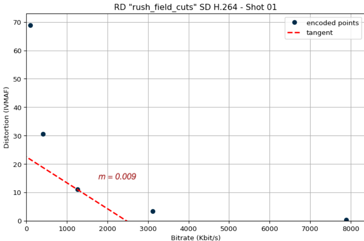
Figure 2.9 , the RD discrete curve of the first shot of rush_field_cuts , with the five encoded points and the tangent to the curve whose slope is closest to sequence_slope .
