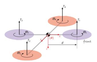
Figure 2.4: Dynamic modelling of a Quadrotor [5]
