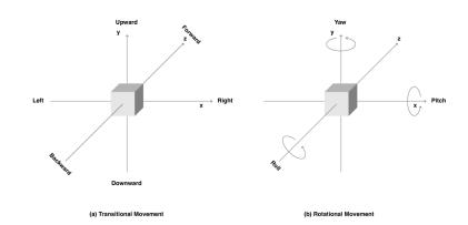
Figure 2.3: Degrees of freedom of an UAV
