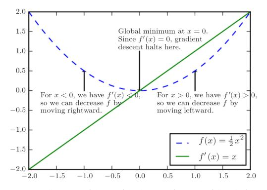
Figure 2.13: Illustration of the use of the derivative function to follow the function to a minimum [11]
