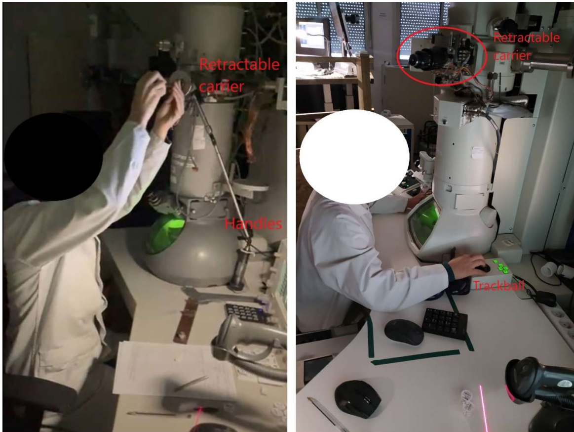
Figure 51: On the left the insertion of the grid carrier into the old MET, while on the right the new MET
