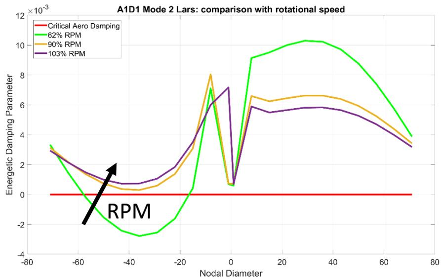
**Figure 81: Aerodamping A1D1 Mode 2: Comparison with rotational speed**
