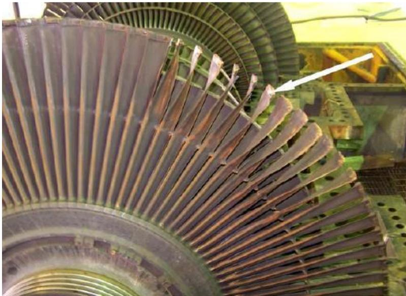
**Figure 25: Flutter damage in a steam turbine [5]**
