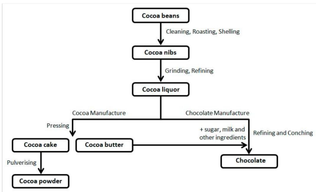
Figure 3 - Flow chart representing the industrial process of the chocolate production. (source: NIH)
