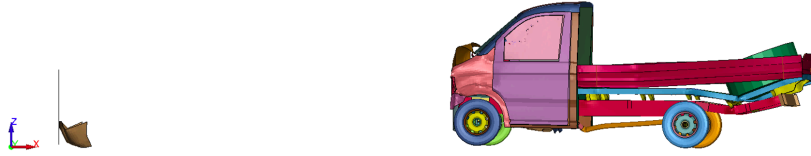
Figure 48. Backward acceleration testing: model with rigid tires and suspensions at t=1 s
