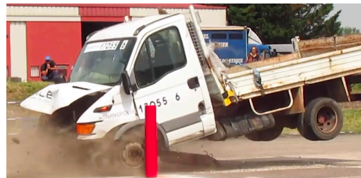
Figure 66. Bollard impact: 45° view
