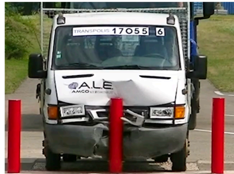
Figure 65. Bollard impact: front view
