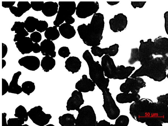
Figure 25. Micrograph of sieved AlSi10Mg powder in acrylic resin
