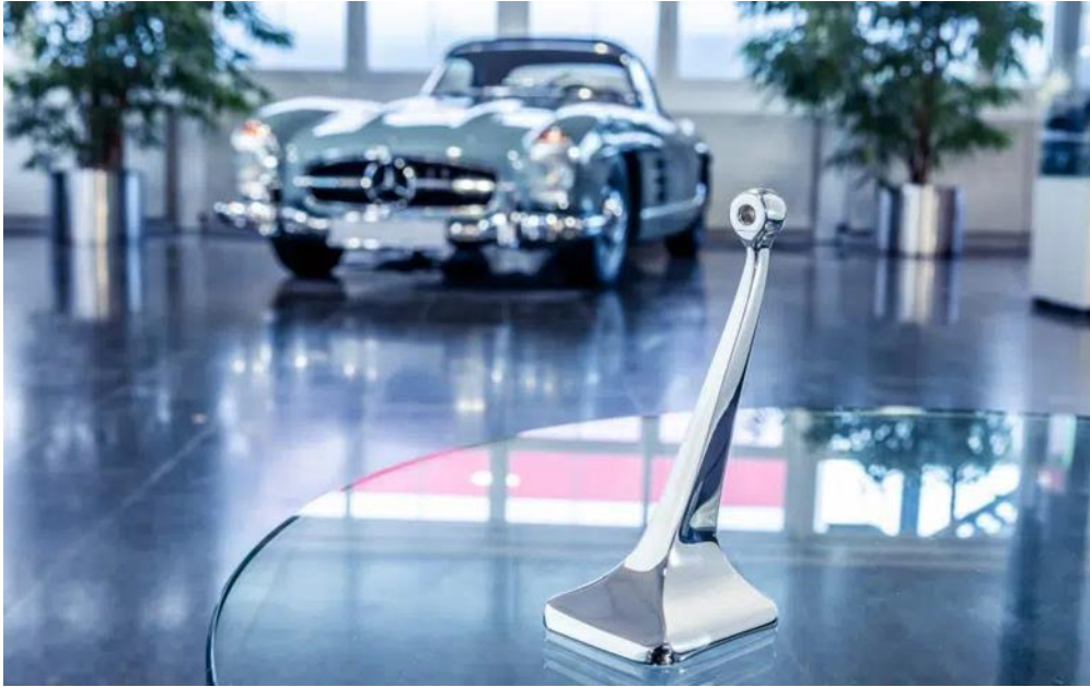
Figure 7 - Component of Mercedes 300SL restored through Additive Manufacturing [25]
