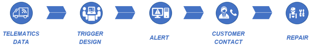
Figure 10 Control Room Process
