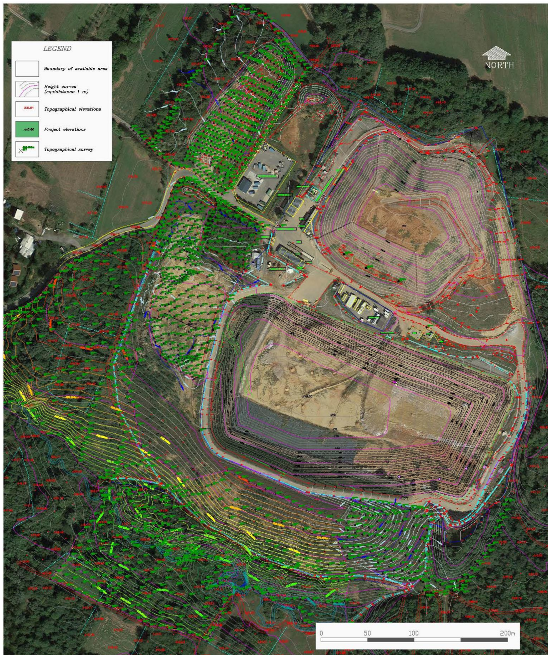
Figure 22: DTM of the area around the landfill. The level curve are in pink lines and the dark crosses are the point of the topographic survey.
