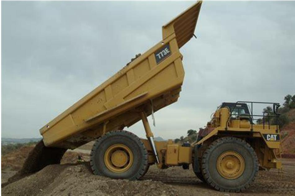
*Fig. 60 - Use of a dumper on the construction site*
