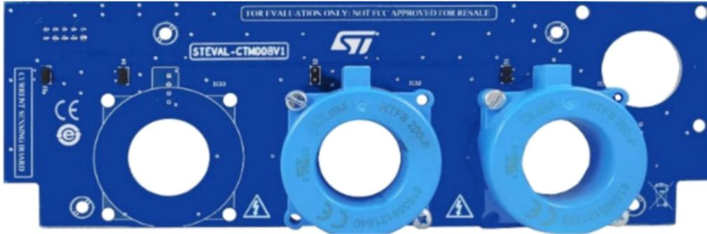
Figura 5.8: STEVAL-CTM008V1 current sensing board[9].
